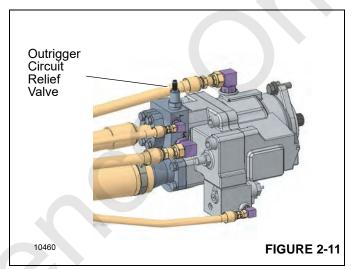
This can be adjusted by first removing the adjustment cover plug using a 3/4 in. allen wrench and using a 3/16 in. allen wrench to adjust the setting. Clockwise rotation increases the setting and each turn gains 61 bar (884 PSI). Be sure to re-tighten the adjustment cover to 5 N·m (4 lb-ft) when setting is correct.
