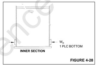
**3.** Measure the thickness of the wear pads and record (twp).
