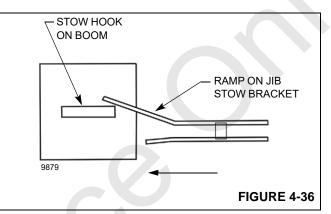
4. Observe the alignment of the front jib mounting bracket on the base boom section and the mounting slots on the jib. If necessary, adjust the vertical and horizontal positions of the front jib mounting bracket as follows:
