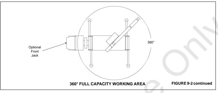
The mounting configuration shown is based on an 85% stability factor.
