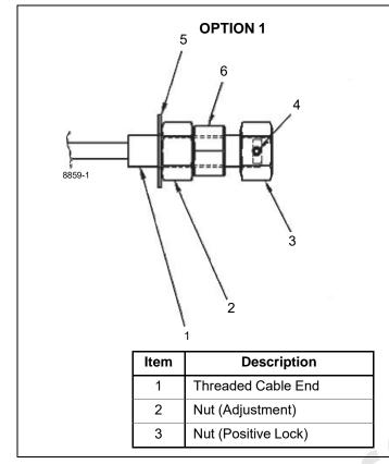
Nut configuration (see Figure 4-23) will be First Nut (ADJUSTMENT) and Second Nut (TORQUED).
