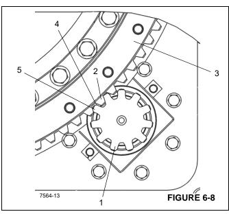
**NOTE:** If a new bearing (3) (Figure 6-8) is installed, a new pinion gear (1) must also be used.
