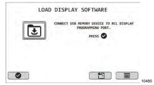
7. Press the vertex key to start the software upload.
