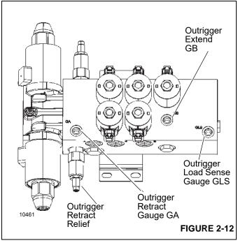
This can be adjusted by first loosening the 0.75 inch jam-nut and using a 0.25 inch Allen to adjust the setting. Clockwise rotation increases the setting and each turn gains 25.5 bar (370 PSI). Be sure to re-tighten the adjustment cover to 8.1 Nm (6 lb-ft) when setting is correct.
