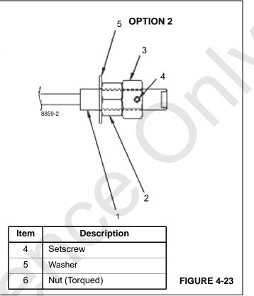
Hold the first (adjustment) nut stationary and a torque wrench to tighten the second (torqued) nut against the first (adjustment) nut to the values indicated in TORQUE VALUES for Second Nut:
