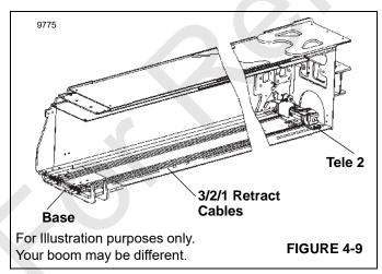
The 3/2/1 retract cables (Figure 4-9) directly oppose the synchronizing cables (Figure 4-8) to ensure that the Tele 1 and Tele 2 section booms extend and retract equally at all times.
