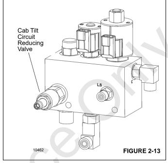
This can be adjusted by loosening the 0.75 inch locknut and using a 0.25 inch hex wrench to adjust the setting. Clockwise rotation increases the setting, and each turn gains approximately 7.6 bar (110 PSI). Be sure to retighten the 0.75 inch locknut to 8.1 Nm (6 lb-ft) when setting is correct.
