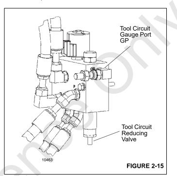
This valve can be adjusted by loosening the 0.75 inch locknut and using a 0.25 inch Allen to adjust the setting. Clockwise rotation increases the setting and counterclockwise decreases the setting. Be sure to retighten the 0.75 inch locknut to 8.1 Nm (6 lb-ft) when setting is correct.
