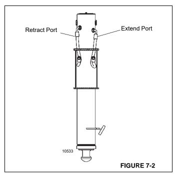
5. Install the fittings in the cylinder, then connect the hydraulic hoses to the jack cylinder as marked prior to disassembly.
