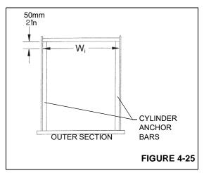
2. The top rear wear pads also act as the top side pads. Each pad is held in position by a retainer plate which is adjusted by way of a cam plate. The retainer plates and cam plates attach to the inner boom top plate. Adjust the left and right cam plates to obtain a total of 2.00 mm (0.08 in) clearance between these wear pads ( $W_o$ ) and inside width ( $W_i$ ) of outer section; adjust the left and right wear pads such that they extend past the inner boom side plates equally.
