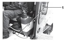
Fig. 59 Safety lever released (pushed forward)
