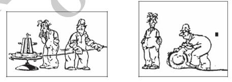
A wire rope supplied on a coil unwound by turnable or an the ground.
