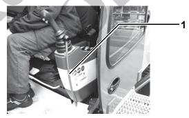
Fig. 58 Safety lever activated (pulled back)
