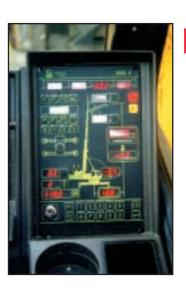
EKS4 electronic load moment indicator operates in conjunction with ECOS continuously displaying crane configuration and load moment data
