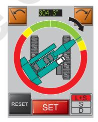
(3) Swing to right direction further and the tip of boom in the swing area limit indication enters into warning area (Yellow), intermittent buzzer sound is issued.
