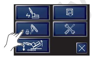
Work area limit setting screen is displayed. (The screen example is crane case.)
