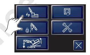
(3) Crane attachment select screen is displayed. Select "9 (Self removal cylinder)".
