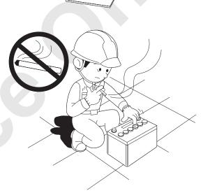
Disconnect the battery cables during inspection and maintenance of electrical system.
