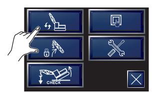
(3) Crane attachment select screen is displayed. Select "10 (Self removal mode)".
