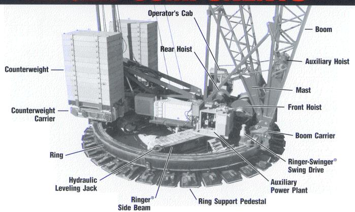
Ringer® Side Beams: High-strength beams connect ring to basic crane. FACT™ connectors simplify set-up. Beams provide mounting for four hydraulic jacks that level the ring during set-up.
