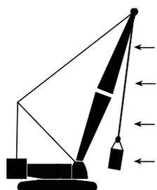
Backward stability is affected by wind on the front of the boom and luffing jib. This condition is especially dangerous when the boom and/or luffing jib is at or near the maximum angle when operating without load.
