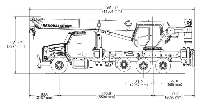
The configurations are based on the NBT40–2 with an 85% stability factor. The complete unit must be installed in accordance with factory requirements and a test performed to determine actual stability and counterweight requirements since individual truck chassis vary.
