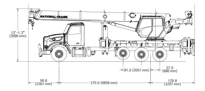
The configurations are based on the NBT45–2 with an 85% stability factor. The complete unit must be installed in accordance with factory requirements and a test performed to determine actual stability and counterweight requirements since individual truck chassis vary.
