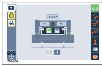
Using the ODM keypad or jog dial, highlight the down arrow
