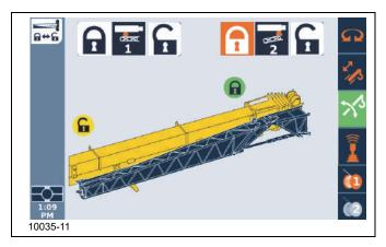
16. Make sure the ODM shows that the front mounting pin (Pin #2) is extended. Visually confirm that the front mounting pin is securely installed. Lock the handle (1, Figure 5-39) with pin (2).
