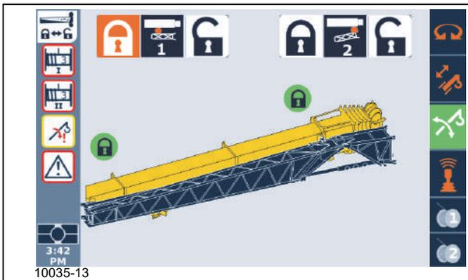
15. Visually confirm that the front boom extension pin (Pin #2 in the ODM) is locked. The handle should be in the up position. When the handle is in the up position, the front mounting pin is extended and the boom installation pins are unlocked.
