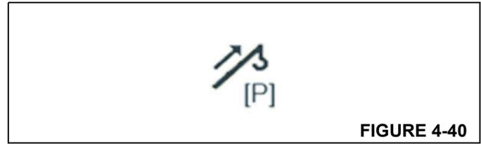
**Semi-auto Mode Telescoping Function Shut-down**
