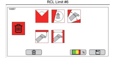
The RCL Limit #6 screen enables the operator to delete all limit values that exist.
