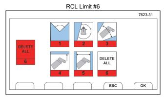
The RCL Limit #6 screen will allow the operator to delete all limit values that exist.
