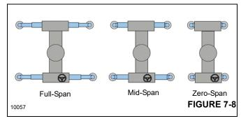
Least common outrigger position determines the chart that is to be used. For example:
