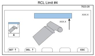
Move the crane boom to the desired boom tip height point (it will appear on the display screen) then select the following:
