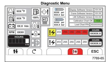
The Diagnostic Menu screen is divided into five different displays that provide software version and revision, crane and truck operating information and warnings, an hour meter, fault code displays and lift cylinder pressure readings.
