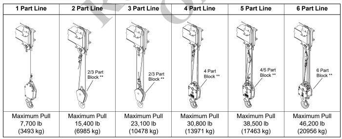
7 Part Line (not shown) uses a 7/8 part block\*\*, maximum pull 53,900 lb (24449 kg)
