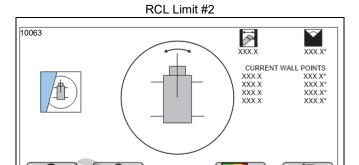
There can be up to four set points which form 3 virtual walls. The points are taken from the rope fall length, radius, and slew angle.
