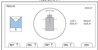
Rotate the crane superstructure to the desired position (the number will appear on the display screen) then:
