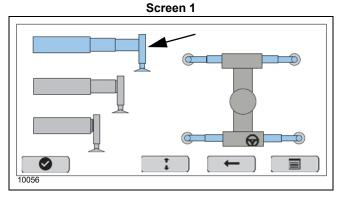
The current outrigger status is displayed by highlighting the current outrigger setting in light blue, shown on the left side of Screen 1. The non-current span setting will be shown in gray.
