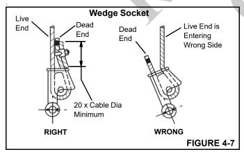
**4.** Loop the cable around the wedge and insert the dead end back into the socket. Pull on the live end until the
