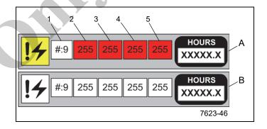
Active Fault Box (Red, A) - The crane control system will display up to 20 active faults or errors in the crane and RCL control system(s). Fault numbers only show when a fault occurs and clears when the fault is corrected. The three digit numbers correspond to a specific fault for a specific module, connector and pin.
