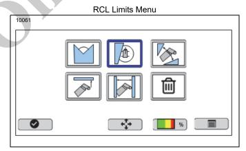
Select the desired operational limit 1 through 6, use the arrow key to the correct operational limit, then select the check mark to select it.
