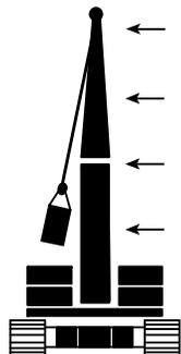
Boom and jib strength is affected the most when the wind acts on the side of the boom and jib.
