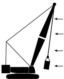
Backward stability is affected by wind on the front of the boom and jib. This condition is especially dangerous when the boom is at or near the maximum angle when operating without load.
