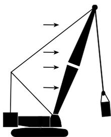
Forward stability is affected by wind on the rear of the boom and jib. Wind applies a force to the boom, jib, and load that adds to the crane's overturning moment. This action has the same effect as adding load to the hook.
