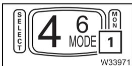
You can also increase the braking force of the engine by switching to the **P (1)** driving mode.
