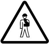
**Danger of overturning when slewing with an incorrectly set RCL!**
