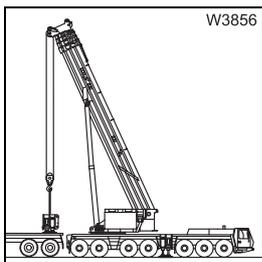
4. Sling the rear outrigger box to the truck crane and lift it from the separate vehicle or from the support; ▶▶▶ *Slings points of the rear outrigger*, p. 6 - 42
