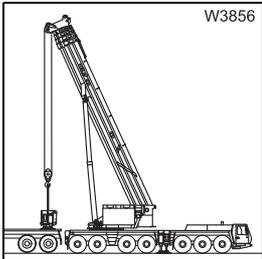
4. With the RCL set correspondingly, unrig the rear outrigger beam;
