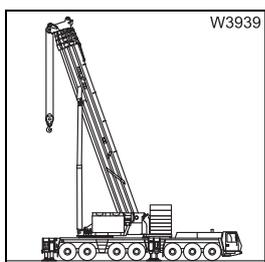
5. Turn the superstructure to the rear and lock it in place;
