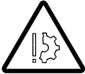
**Danger! Body parts could be crushed when establishing a connection for the suspension.**
