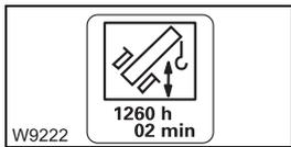
You can display the operating hours of the derricking gear;
