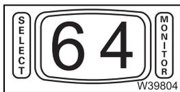
– The currently selected gear is displayed (e.g. 4th gear) and the transmission is set to locked position.
