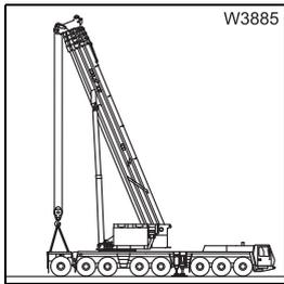
**10.** Sling the additional axle to the truck crane; *Slingsing points on the additional axle, p. 6 - 96.*
