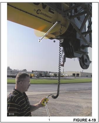
**10.** Use the controller to pivot the boom extension so that lugs (1, Figure 4-20) on boom extension align with the holes in the lugs (2) on the boom nose.
