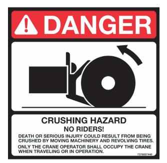
**Do not remove** the *Load Chart*, this *Operator Manual*, or any decal from this crane.
