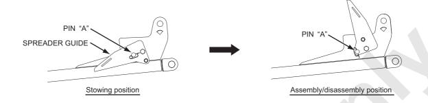
(B) Lower the boom. After the tip end of the boom has been grounded, slowly loosen the boom hoist wire rope more. The spreader is lowered along the spreader guide. When the hole of the spreader is aligned with the pin hole of the bracket on the boom base section, insert pin "B" to connect the spreader to the base boom bracket.
