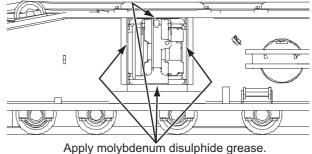
(2) Take out the clearance adjusting shims between the crawler and the axle.
