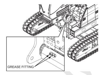
Supply grease to the boom drum lock from the grease fitting provided under the swing frame.
