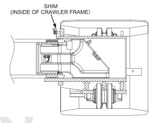
(6) Take out the pin "N" which has connected the crawler ext/ret cylinder and the crawler and retract the cylinder fully.
