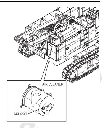
The engine air cleaner is clogged. Clean or replace the element.
