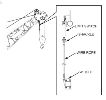
4. Pass the front drum wire rope through the hook (s) and boom point sheave (s) in order. Fix the wire rope end to the boom point for even number part reeving and to the hook for odd number part reeving with the rope socket.
