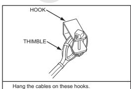
Hang the cables on these hooks. Otherwise undue force would be applied on the hook limit connector. Ensure to hang thimble on these hook.
