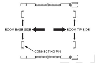
2. Connect the prepared guy lines from the boom tip side to the basic machine side one by one.
