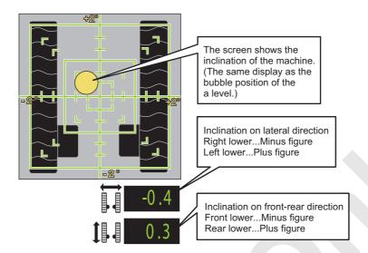
The above figure indicates example of condition that right rear part is lower.
