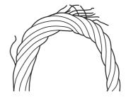
Bend rope sharply to expose breakage.
