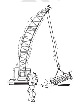
20. Trying to lift a load which is stuck, frozen or attached to something else may result in tipping, boom collapse or other damage. Be sure that loads are free before lifting.
