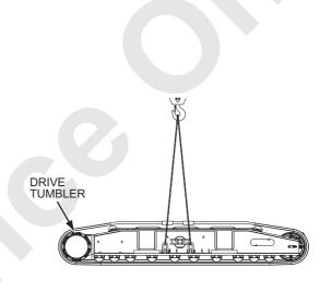
In case of using an assisting crane, remove with the procedure as shown right.
