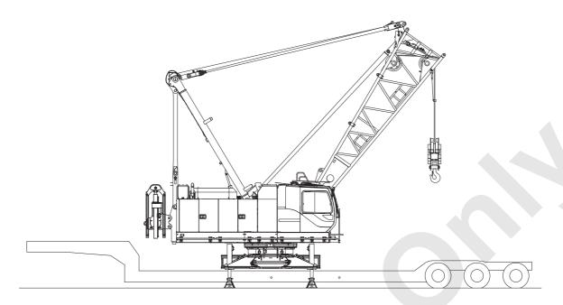
(12) Lift the main machinery further up and let the trailer go out under the main machinery.Effective gap of the main machinery:1,093 mm (3' 7")
