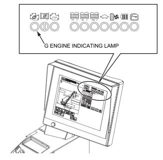
\* When the above warning is issued, lower the lifting load and turn OFF the key switch.
