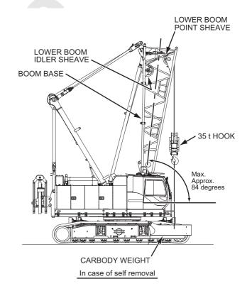
(B) Install the "a" area of the carbody weight to the "b" area of the carbody.
