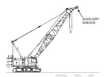
Lift the auxiliary sheave with the assisting crane. Secure it to the boom top with the pins and lock them with spring pins (2 positions, both upper and lower sides).
