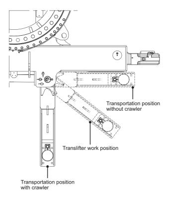
(8) By controlling the crawler extend control switch of the remote controller, extend both crawlers (right and left) toward outside.
