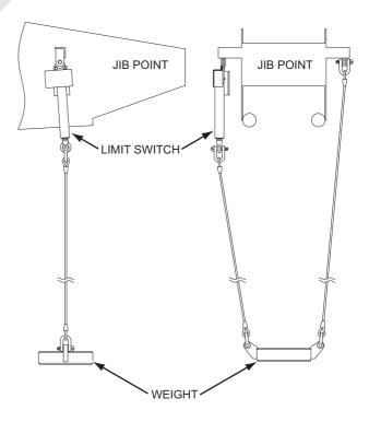
4. Pass the wire rope end through the weight for the limit switch, and secure the end to the hook rope socket with the bolt, nut and split pin.
