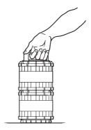
(2) Hold the top mold plate and loosen the grip.
