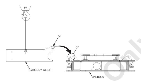
(C) Insert the carbody weight installation pin "A" and secure it with the lock pin "B".
