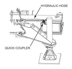
(3) Remove the pin "C" as shown right and remove the float from the vertical cylinder. Load the float on the trailer and secure them to prevent falling off the trailer.
