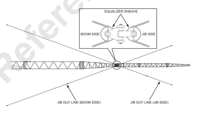
5. Connect both ends of the jib guy line to the top end of the jib.
