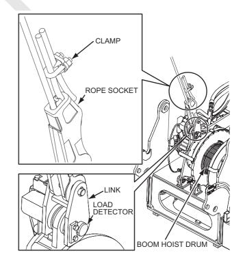
(3) Wind up the wire rope to the boom hoist drum slowly by turning the boom drum control lever to raising side.
