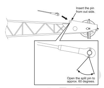
6. Install the jib guy line link to the boom insert with lug, referring to the "Boom and guy line configuration chart".
