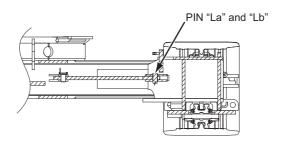
(2) Hold the left crawler, use corner protection materials so that wire does not bite into shoes. Refer to P.8-7 [WEIGHT AND DIMENSION IN DISASSEMBLY] as for one side crawler weight.
