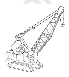
23. Trying to repair or adjust equipment with a suspended hook or load or with the boom raised could release machinery and let it move unexpectedly.
