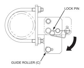
3. Take out the roller of the guide roller (C) to the work position and secure with the lock pin.
