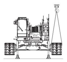
(4) When both crawlers are installed completely, hold the main machinery horizontally and retract the four vertical cylinders until the crawlers are placed completely on the ground.
