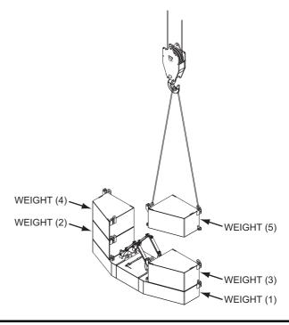
5. Secure right and left counterweights with the connecting pins respectively and retain them with the spring pins. (8 locations)
