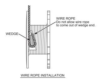
(2) Pull the boom hoist wire rope manually and tap lightly on the wire rope to align and wind the wire rope slowly.
