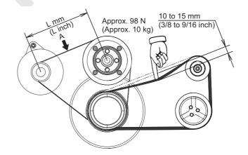
Checking method of tension
