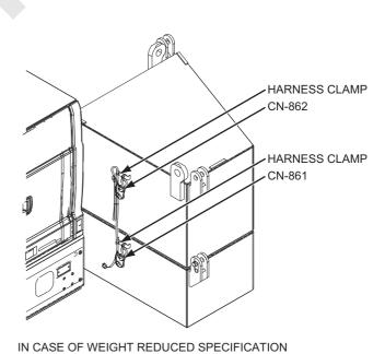
In setting the LMI, ensure to select the item matched with the actual weight condition. If unmatched item is selected, error [ML-ME063] would be displayed in the monitor and the buzzer would sound.
