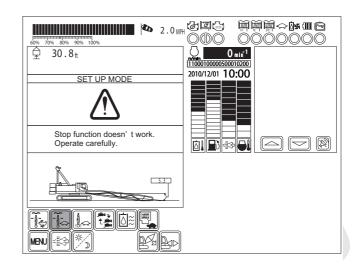
STOP RELEASE MODE WHEN TRANSPORTATION WITH BOOM BASE ATTACHED. (ONLY MACHINE WITH REDUCED WEIGHT SPECIFICATION)
