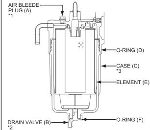
\*1 Referenced tightening torque: 8 to 12 N-m
