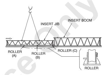
2. After the jib insert has passed the rollers (A), move them to the front of the jib insert.
