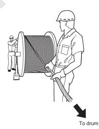
Kink: Deformation by twisting of wire rope
