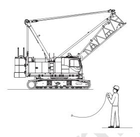
(10) If the counterweight quantity detect unit is equipped, connect the detect harnesses installed on all of the counterweights and the main machinery harness.
