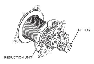
FRONT, REAR DRUM MOTOR AND REDUCTION UNIT
