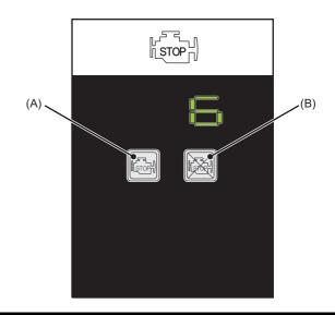
When the engine is stopped due to the auto idle stop function, the engine can be restarted by turning the accelerator grip.
