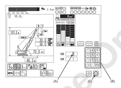
Layer number can be checked by measuring distance from drum flange step and the wire rope.
