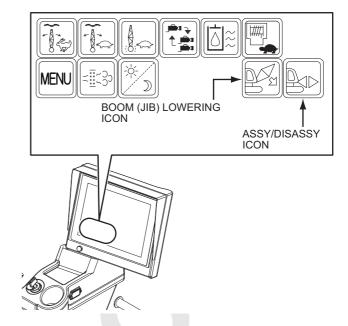
5. By lowering the boom further, the hook overhoist limit switch operates when the weight of the hook overhoist limit switch is placed on the ground, and the boom lowering is automatically stopped again. Press and hold the "Assy/disassy" icon one time for approx. 1 second and it becomes the Assy/disassy mode, and the boom can be lowered. Be careful because the hook overhoist automatic stop does not function in the Assy/disassy mode.
