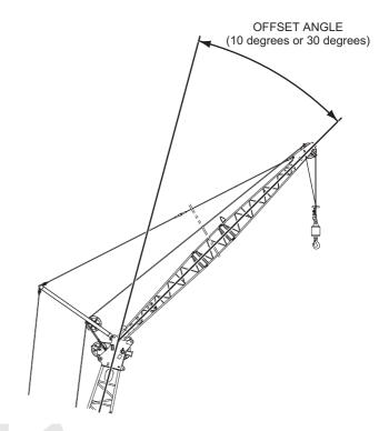
4. Temporarily remove the equalizer sheave of the jib strut, and pass the jib guy line through the sheave. Only then, reinstall the sheave back to the original position (keep the strut down).
