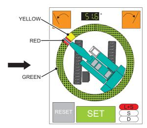
(C) Swing the crane to the place just before the obstacle on the right side and stop and push the icon [RIGHT LIMIT POSITION SET]. The crane figure swings to right. Push [RIGHT
