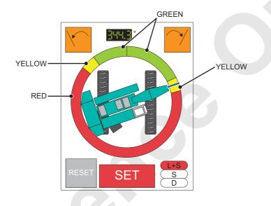
(4) If the crane continues to swing further and the front of the boom enters into red area on circle, continuous warning sound is issued and swing motion stops.
