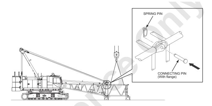
(3) Lift up the connecting section of the boom base and the boom insert and align the bottom connecting pin holes, and insert the connecting pins (double tapered pin) into these holes. Insert the spring pins into the connecting pins to fix them.
