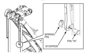
e. Insert the pin "Y" into the gantry and retain with the spring pins.
