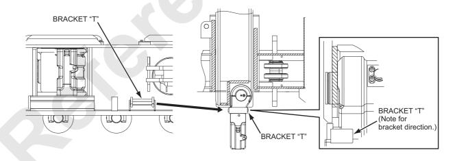
(5) Take out the clearance adjusting shims between the crawler and the axle.
