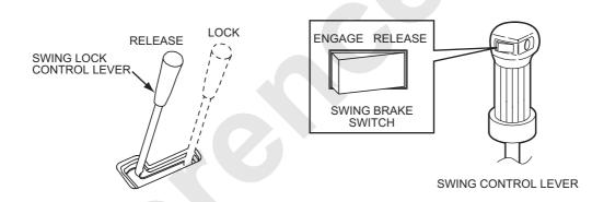
Push the swing control lever forward to swing the upper to the left and pull the lever backward to swing the upper to the right.
