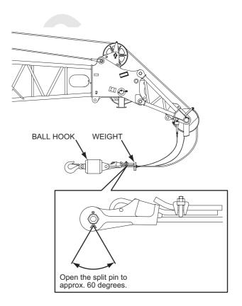
5. CONNECTING THE LOAD SAFETY DEVICE
