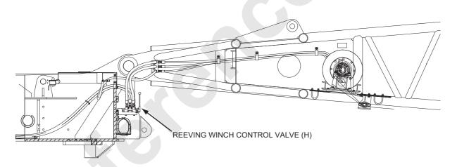
4. Connect the hoses from the reeving winch control valve (H) to the piping block (J) on the boom base left side with each hose coupler (E) (F) (G). Connect each hose coupler so that the male and female fitting of the piping block (J) match each other.
