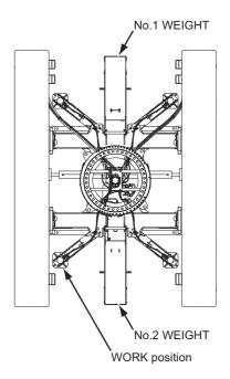
There are two ways to remove the carbody weight. One is to use an assisting crane and the other is to use the machine boom base.
