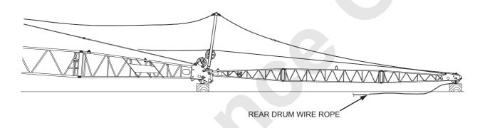
3. Install the hook overhoist limit switch and weight to the jib point section.
