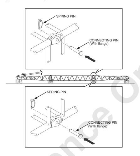
2. Lift up the preassembled jib with the assisting crane connect it to the boom point section.
