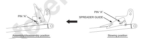
(2) By following the procedure (B) in "HOW TO USE SPREADER GUIDE" connect the spreader and the boom base bracket with the pin "B". Then remove the guy line connecting pin and remove the base guy line from the upper spreader.
