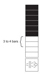
Auto regeneration becomes actuated when control lever is not used and burning (regenerating) soot starts automatically.
