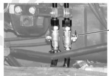
Cab Heater Shut-Off Valves (2) Shown Closed
