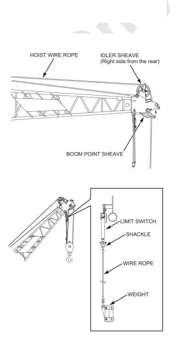
4. Pass the front drum wire rope through the hook sheave(s) and boom point sheave(s) in order. Do no forget to pass the wire rope through the weight for the overhoist limit switch.
