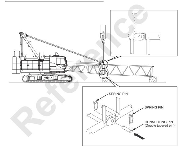
(4) Referring to Boom and guy line arrangement chart, connect the boom inserts in order in the same way.
