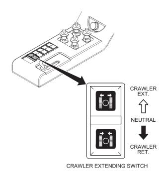
(9) After extending the crawler for approx. 400 mm (1' 4") (Ref: ext/ret stroke is 815 mm (2' 8")), stop the crawler ext/ret switch once and place the pin "L" on extending/retracting side on the link.
