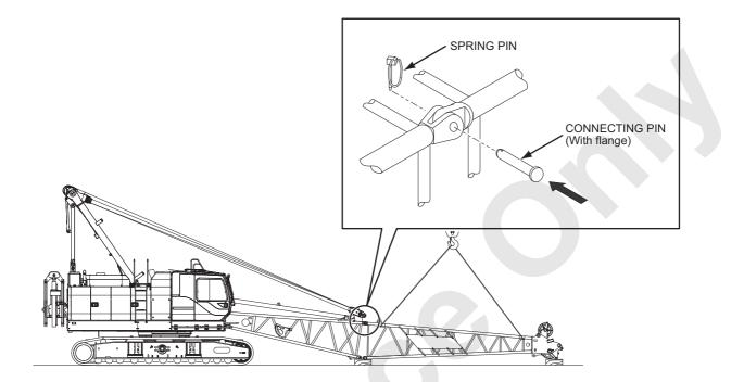
2. Raise the boom base until the lower pin holes are aligned with each other. Then tap the connecting pins (double tapered pin) in, and insert the spring pins into the both ends of the connecting pin.
