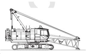
2. Fix the upper spreader to the boom base top bracket with pins.
