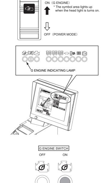
\* When the above warning is issued, lower the lifting load and turn OFF the key switch.
