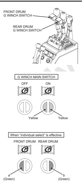
(3) When the individual select lamp is turned ON, preparation is completed. Start each lever control. High speed raising or lowering becomes possible.
