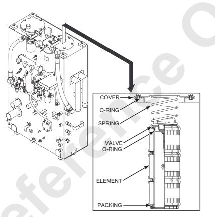
(1) Remove the filter assembly and place it on flat surface.
