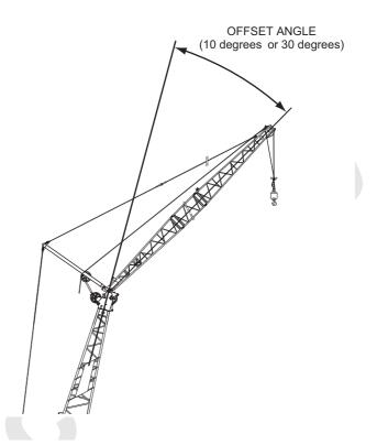
Temporarily remove the equalizer sheave of the jib strut, and pass the jib guy line through the sheave. Only then, reinstall the sheave back to the original position (keep the strut down).
