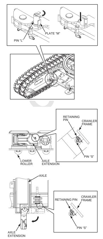
(2) Pull out the pin "S" which secure the axle extension and the crawler frame.
