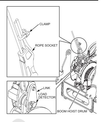
2. INSTALLATION OF BOOM HOIST WIRE ROPE TO THE DRUM
