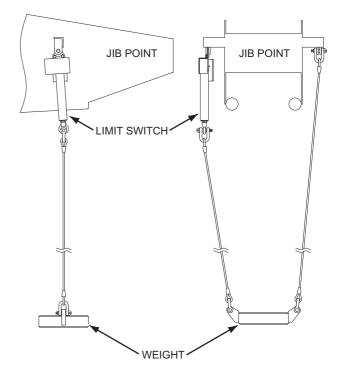
4. Pass the wire rope end through the weight for the limit switch, and secure the end to the hook rope socket with the bolt, nut and split pin.
