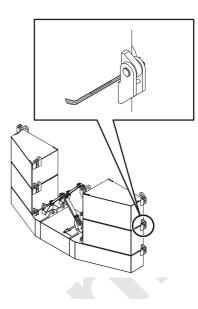
7. Propel the crane to the position where the counterweight link and the base machine counterweight link can be connected.
