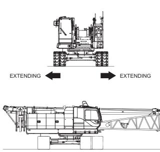
(7) If the crawler cannot be extended with main machinery faces front due to ground condition, swing the upper machinery slowly to right angle with the crawler.
