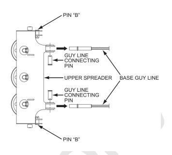
(3) Operate the boom hoist control lever to tighten the boom hoist wire rope to remove load from the bottom connector section, then draw out the bottom connecting pins (both ends of which are tapered).
