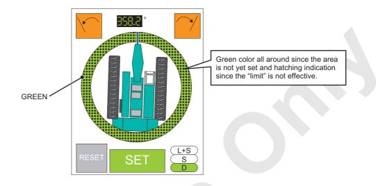
(B) Swing the crane to the place just before the obstacle on the left side and stop and push the icon [LEFT LIMIT POSITION SET].
