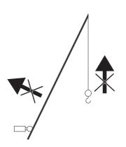
Normally when boom overhoist occurs, controller functions to stop automatically. If auto-stop function is being released and operated, the final stop limit switch control becomes actuated and machine auto-stops. In this case, auto-stop cannot be released.
