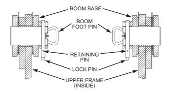
4. Hold the boom base foot area with the assisting crane and pull out the cab side (right hand) boom foot pin first and then left side boom foot pin.
