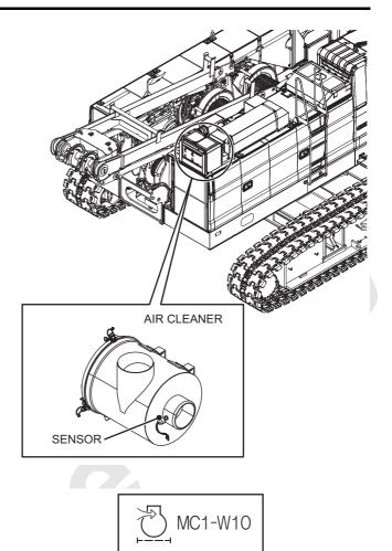
The engine air cleaner is clogged. Clean or replace the element.
