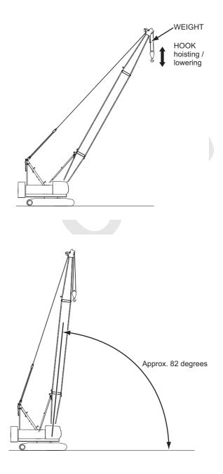
(2) When the boom is raised to approx. 82 degrees of boom angle, boom raising must be auto-stopped.
