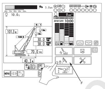
(3) Work area limit setting screen become indicated.(The screen example is crane case.)Push the figure area if new setting is required.
