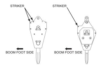
When installing the rope socket to the boom point, pay attention on the side of rope socket. Do not fail to pass the wire rope through the hook overhoist limit switch weight.
