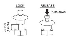
These knobs are to lock the drum for safety during lowering the lifting load or boom.
