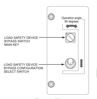
LOAD SAFETY DEVICE BYPASS SWITCH MAIN KEY
