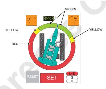
(2) From this condition, if the crane swings to right, crane figure turns right.
