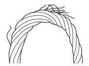
Bend rope sharply to expose breakage.
