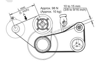
Checking method of tension
