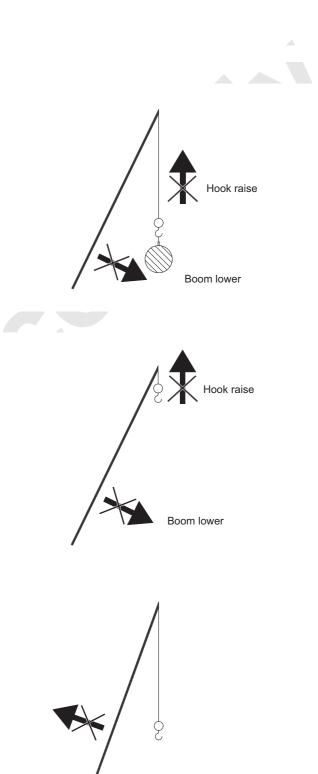
(4) Boom overhoist (Final stop limit switch control)
