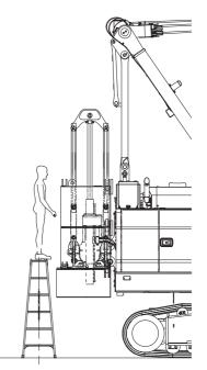
6. Pull out the weight support pin using an extension bar.
