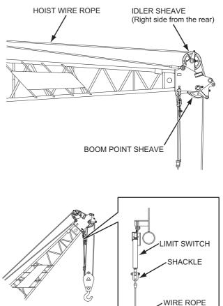
Install the overhoist limit switch and weight to the left side bracket on the tip end of the boom.
