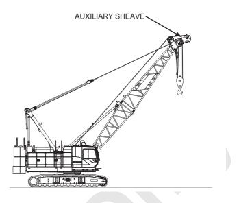
Install the auxiliary sheave installation position at the boom top, and fix it with the pin.
