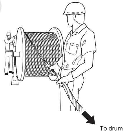
Kink : Deformation by twisting of wire rope
