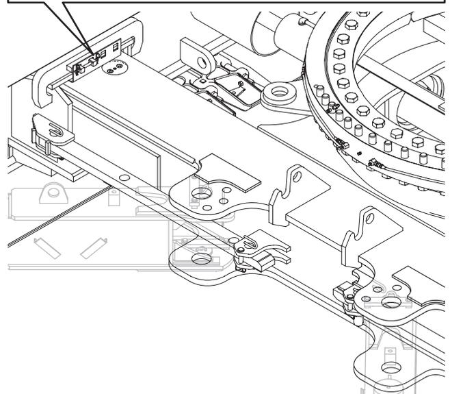
6. Remove the securing pin connecting the crawler ext./ret. cylinder and the crawler frame and retract cylinder fully.
