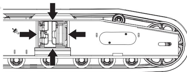
Coat the grease on the sliding surface of axle.
