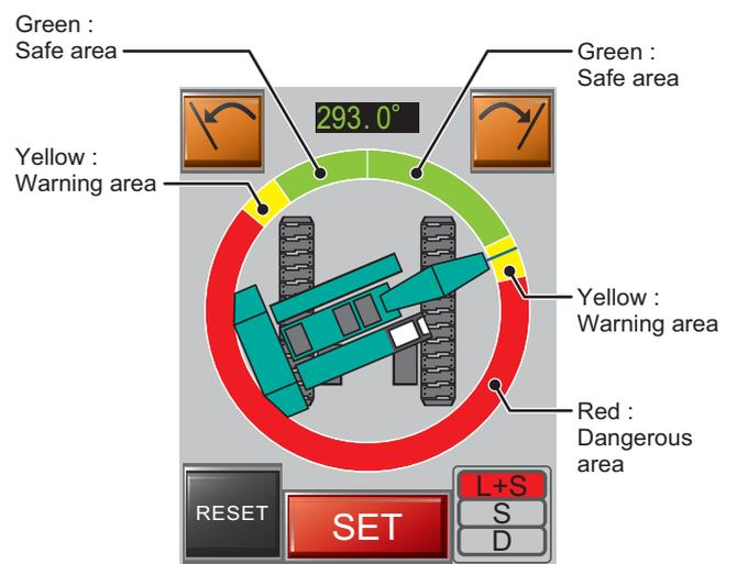
(4) Swing to right direction further and the tip of boom in the swing area limit indication enters into dangerous area (Red), continuous buzzer sound is issued and the swing motion stops.
