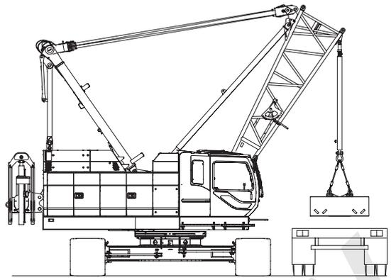
8. Remove the carbody weight (2) as same manner as carbody weight (1).
