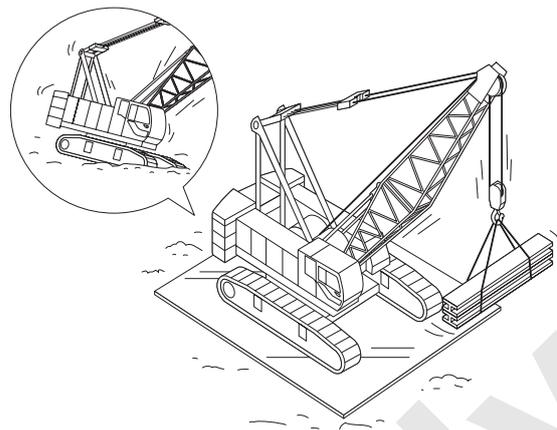
3. The rated capacity of a crane is determined with the crane leveled within  $\pm 0.5$  degrees of grade (1 foot drop or rise in 100 foot distance).
