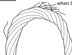
Broken wire may expose when bend the wire rope.
