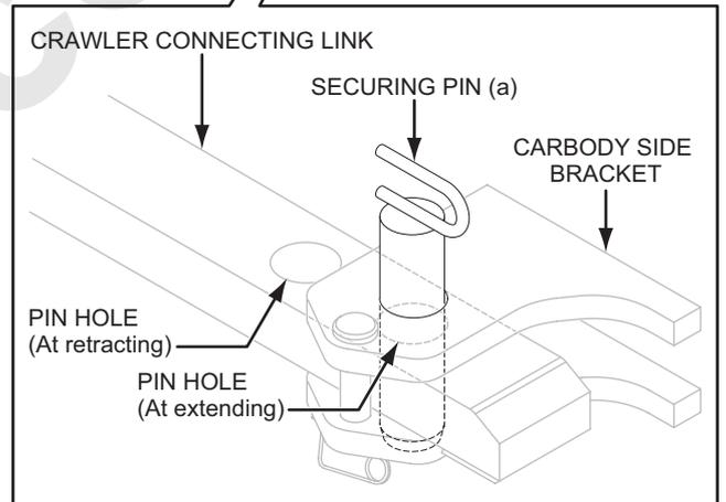
10. In case of extending the crawler by one side, swing the upper machinery 180 degrees and extend the remaining crawler as same order as other side.
