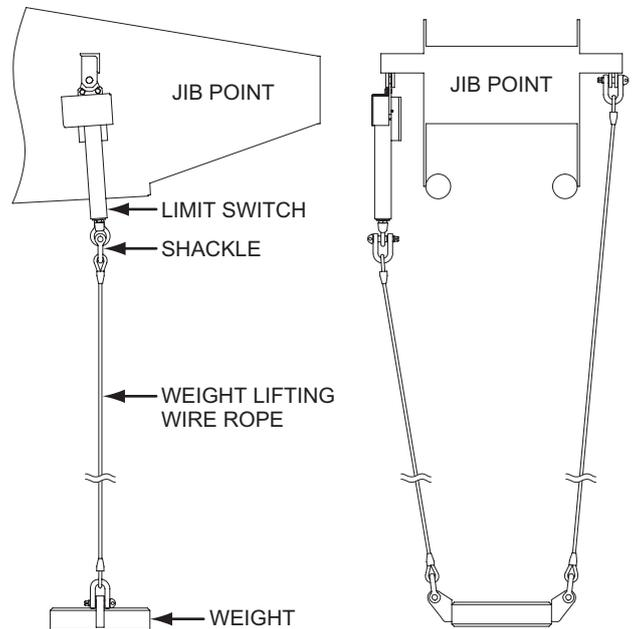
4. Pass the wire rope end through the weight for the limit switch, and secure the end to the hook by the rope socket with the bolt, nut and pin.
