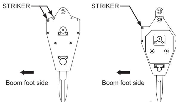
When installing the rope socket to the boom point, pay attention to the direction of rope socket. Be sure to pass the wire rope through the hook overhoist limit switch weight.
