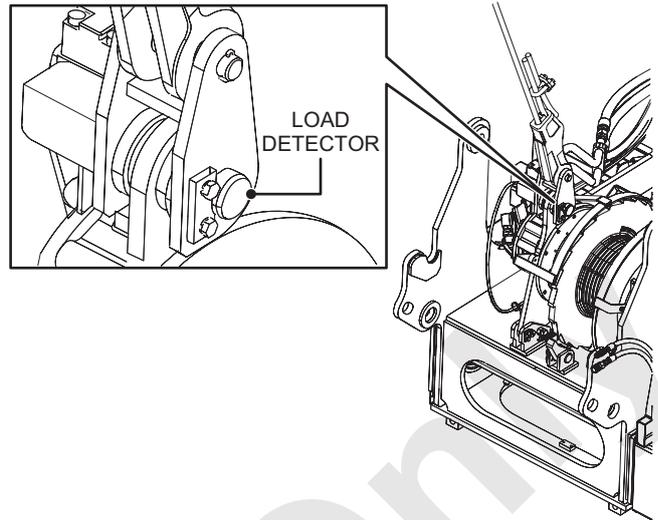
If jib or aux. sheave is not used, connect the hook overhoist limit switch wiring at this time.
