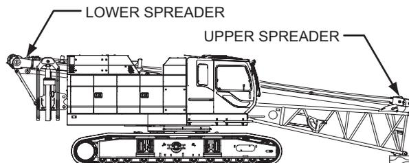
1. Turn the boom drum control lever to lowering side to pay out the wire rope from the boom drum.
