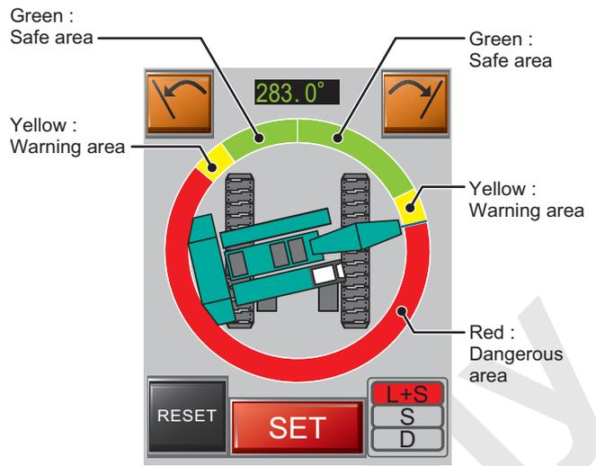
(5) After swing motion stops, swing to safe direction (left) and the tip of boom returns to safe area (Green).
