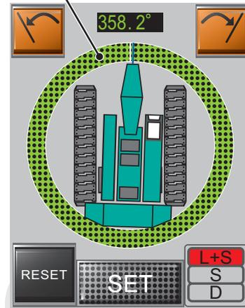
(B) Swing the crane left to the safe place just before the obstacle on the left side and stop.
