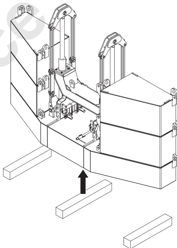
9. Set the counterweight securing pins on both sides with using the extension bar.
