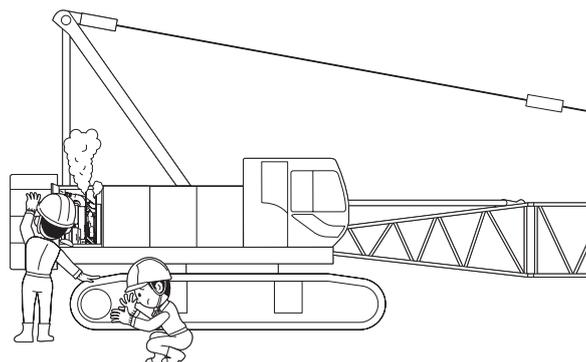
24. Pressure in hydraulic systems can be retained for long periods of time. If not properly released before maintenance people attempt to work on the hydraulic systems, this pressure can let machinery move or cause hot oil and hose ends to shoot out at high speed. Release system pressure before attempting to make adjustment or repairs.
