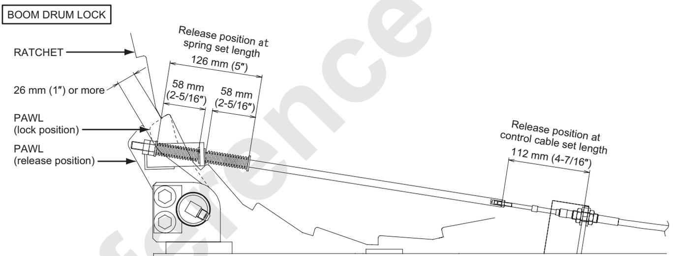
3. Push the drum lock knob in the release position and check to see that the pawl is clear of the ratchet by at least 26 mm (1 in.).
