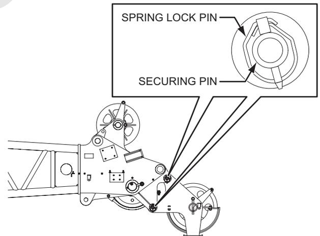
5. Remove the auxiliary sheave assembly from the boom tip.
