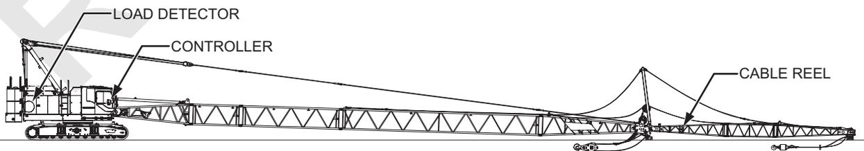
7. Set the crane configuration into the controller (Overload safety device) by referring the article "3.5.1 SETTING OF CRANE CONFIGURATION".
