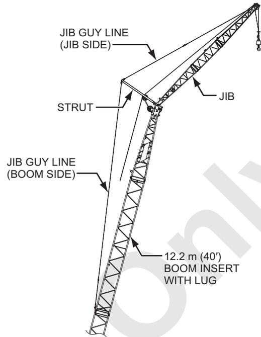
1. Assemble jib and strut on the extension line of the boom tip.
