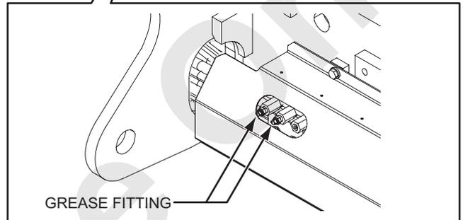
Supply grease to the boom drum lock from the grease fitting provided under the swing frame.
