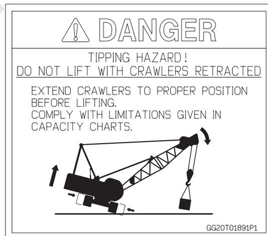
4. If machine swings or is assembled / disassembled with crawler retracted, main machinery may turn over to rear side.
