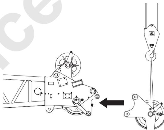
2. Insert the securing pin to secure the auxiliary sheave.
