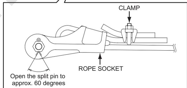
5. Connecting the load safety device
