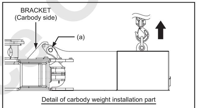
8. Lower the boom slightly and move the carbody weight away from the base machine.
