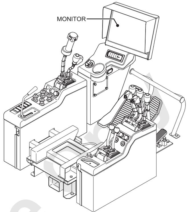
The monitor can be displayed by the selection of monitoring camera equipped at respective locations.
