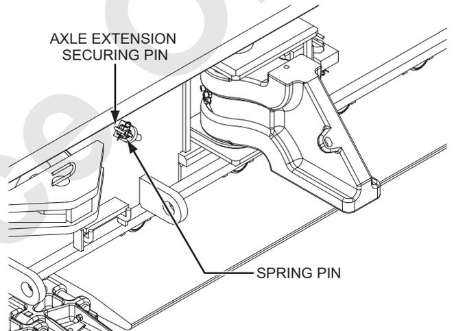
11. Rotate all 4 axle extensions for 90 degrees toward the frame to make them right angle with axles.
