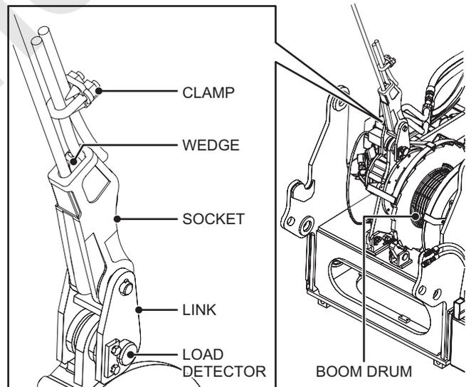
3. Wind the wire rope to the boom drum.
