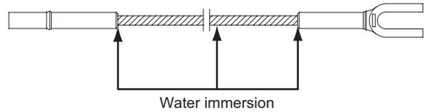
If the internal damage or corrosion is progressed, guy line may be broken and may cause serious accident.
