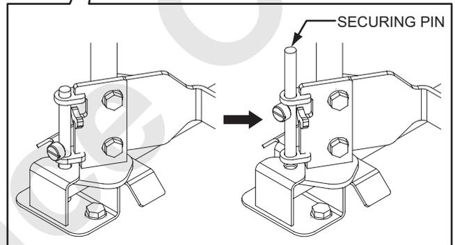
2. Lift up the ladder and remove from the right hand guide.
