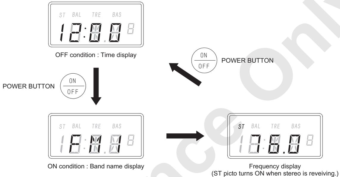
Under this condition, by pressing "DISPLAY SELECT BUTTON" (frequency/time), frequency display and time display alternates.
