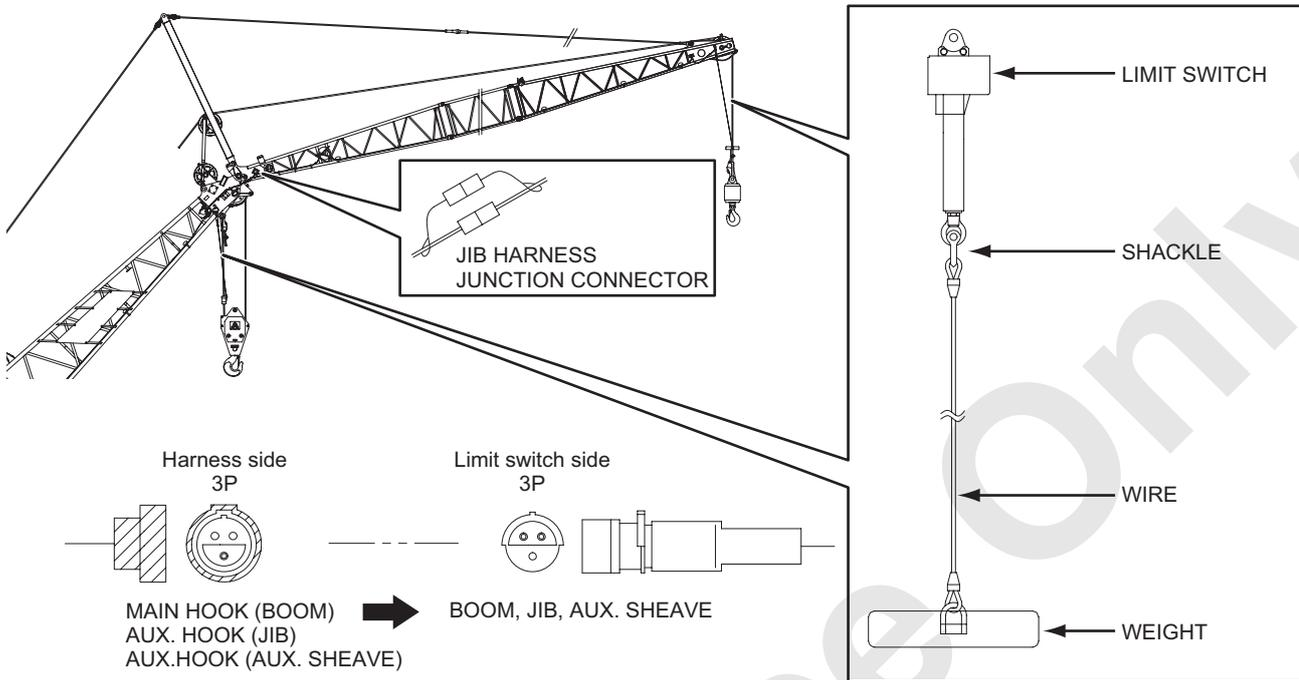
13. LOAD SAFETY DEVICE RELEASE SWITCH
