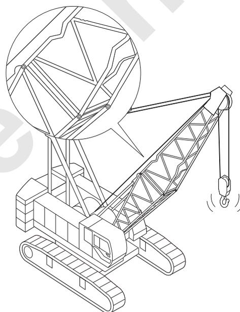
16. Crane booms can collapse if side loaded (pulled sideways).
