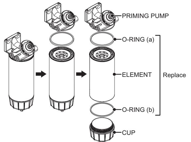
• **Installing the fuel filter element**
