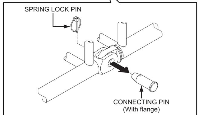
5. Disassembling the boom insert
