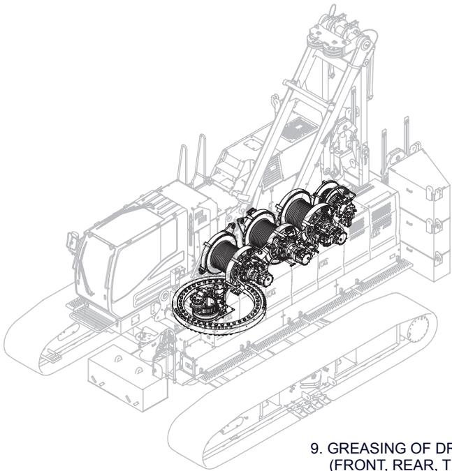
9. GREASING OF DRUM SHAFT BEARING
