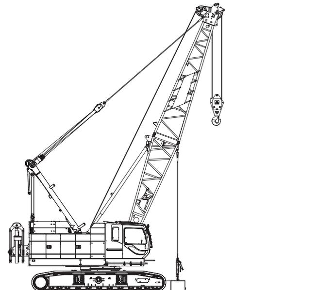
10. Remove the carbody weight (2) as same manner as carbody weight (1).
