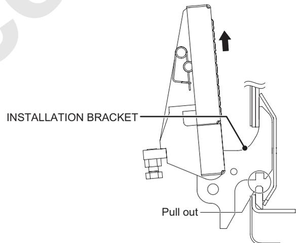
(4) When disengage the securing part, the installation bracket will rotate by its self-weight and remove the step toward to pull closer from the guard.
