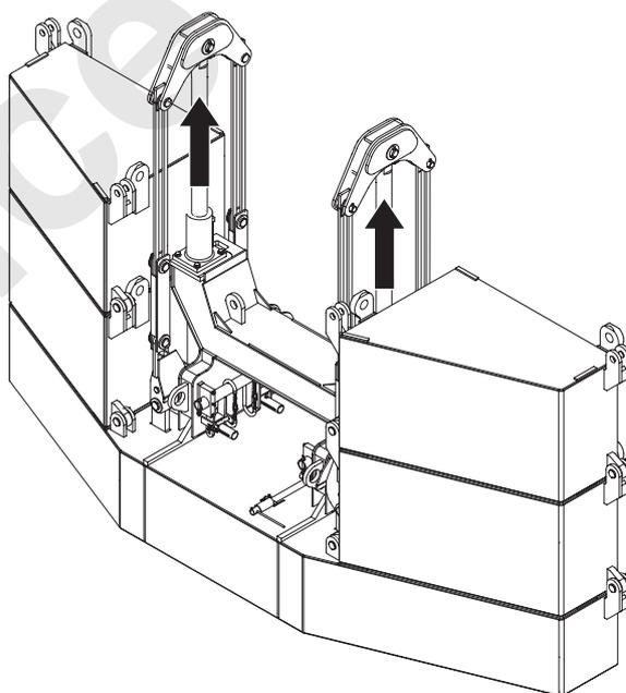
5. Go up onto weight (1) with using the ladder.
