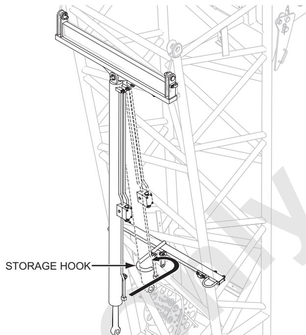
3. Manipulate the self removal cylinder control switch in the operator's cab and retract the cylinder.
