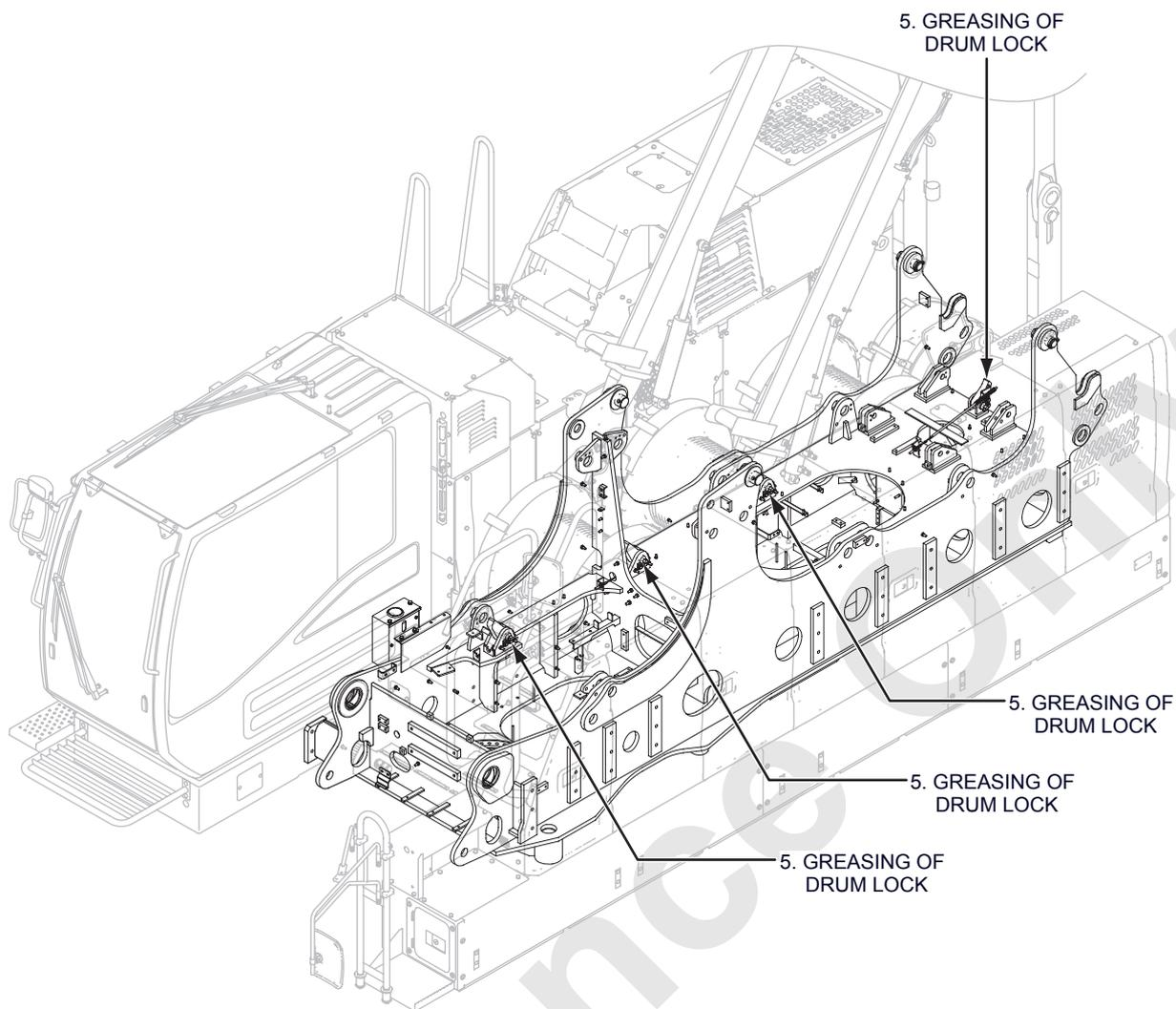
The number in the list below is corresponding to the figure and table on “7.3.4 INSPECTION, GREASING (WATER SUPPLY) ON EACH POINT”.
