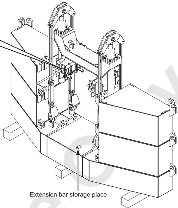
6. Connect the remo-con cable to the connecting portion on the self-removal device.
