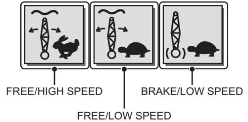
This icon is to select the swing control and swing speed based on work contents.
