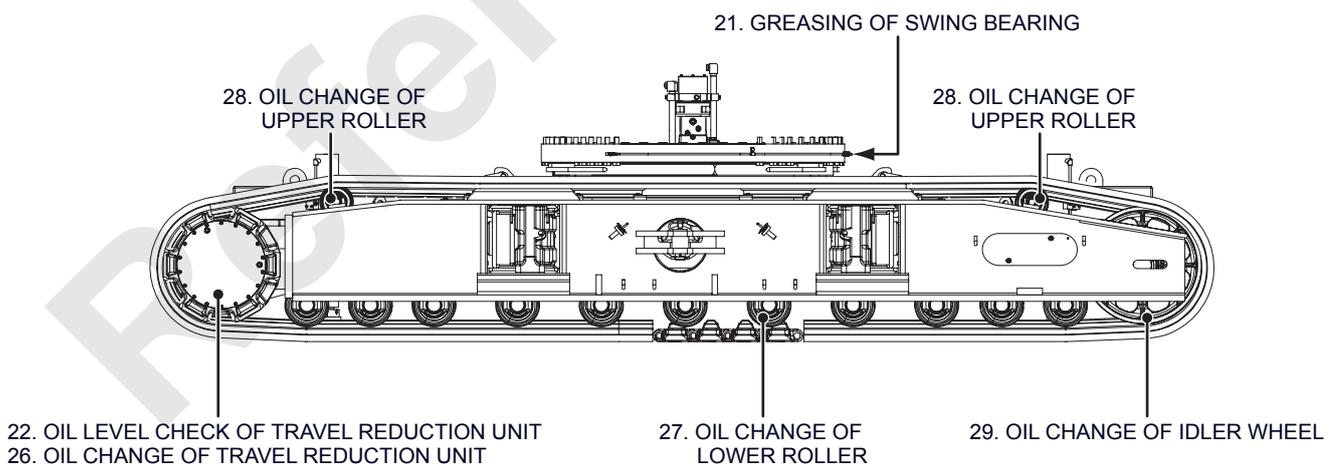
The number in the list below is corresponding to the figure and table on “7.3.4 INSPECTION, GREASING (WATER SUPPLY) ON EACH POINT”.
