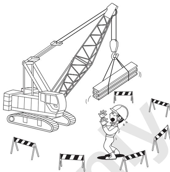
10. Rapid swings or sudden starts and stops can cause the hook and attached load to swing out of control. Always start and stop movements smoothly and swing at speeds that will keep the load under control.
