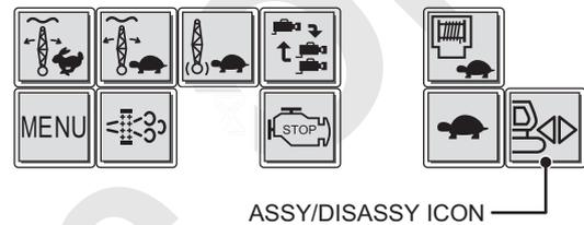
To lower the boom further, return the control lever to neutral then press
