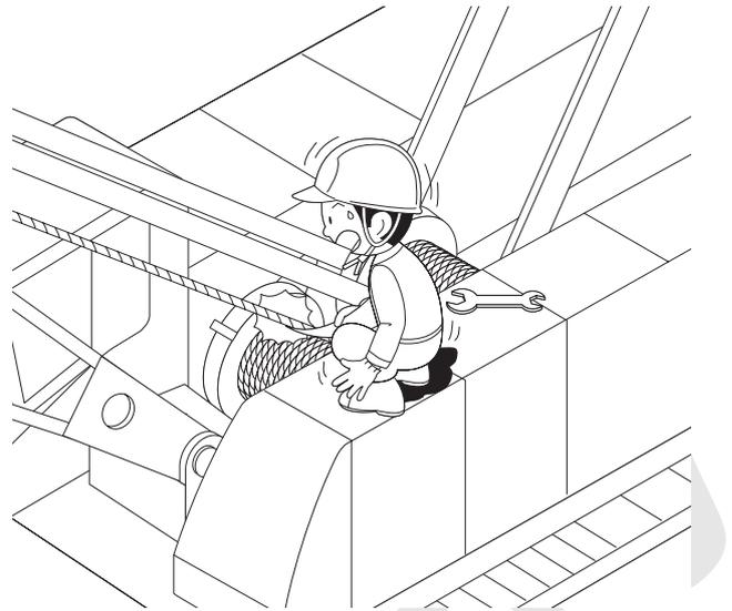
33. The operator should test the winch brakes when a load is first lifted, and when the load is only a few inches above its starting position, to assure the ability of the brakes to hold the load while it is aloft.
