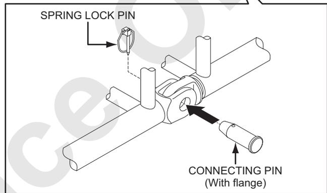
(4) Referring to boom and guy line arrangement chart, connect the boom inserts in order in the same way.
