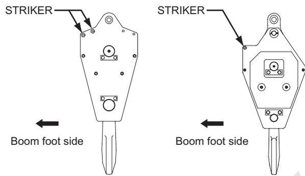
When installing the rope socket to the boom point, pay attention on the side of rope socket.
