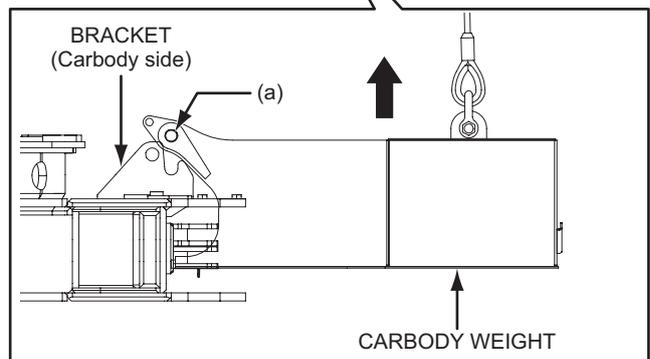
6. Lower the boom slightly and move the carbody weight away from the main machinery.
