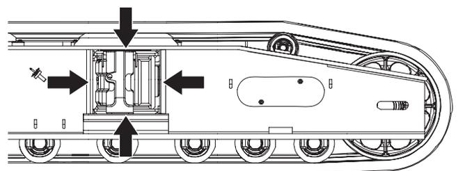
Coat the grease on the sliding surface of axle.
