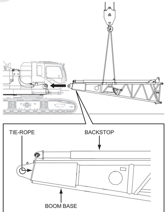
3. Align the boom foot pin hole on both sides and insert the right side pin from inside then the left. Insert the lock pins from top to bottom and fix them with the split pins.
