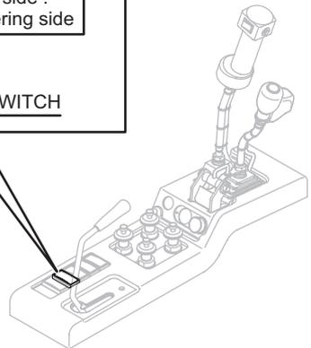
Switch returns automatically to neutral position when hand is released.
