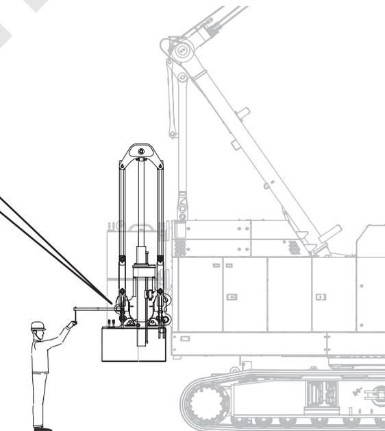
12. Fully retract the cylinders by controlling the remote control switch.
