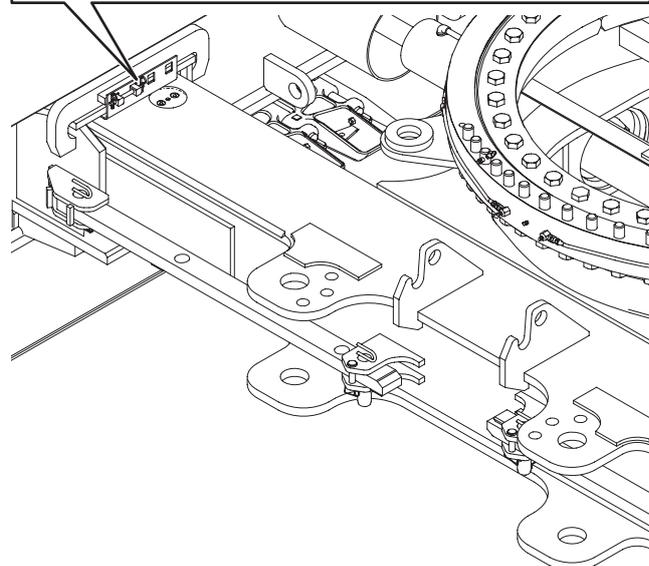
4. Take out the securing pin (a) connecting the carbody and link.
