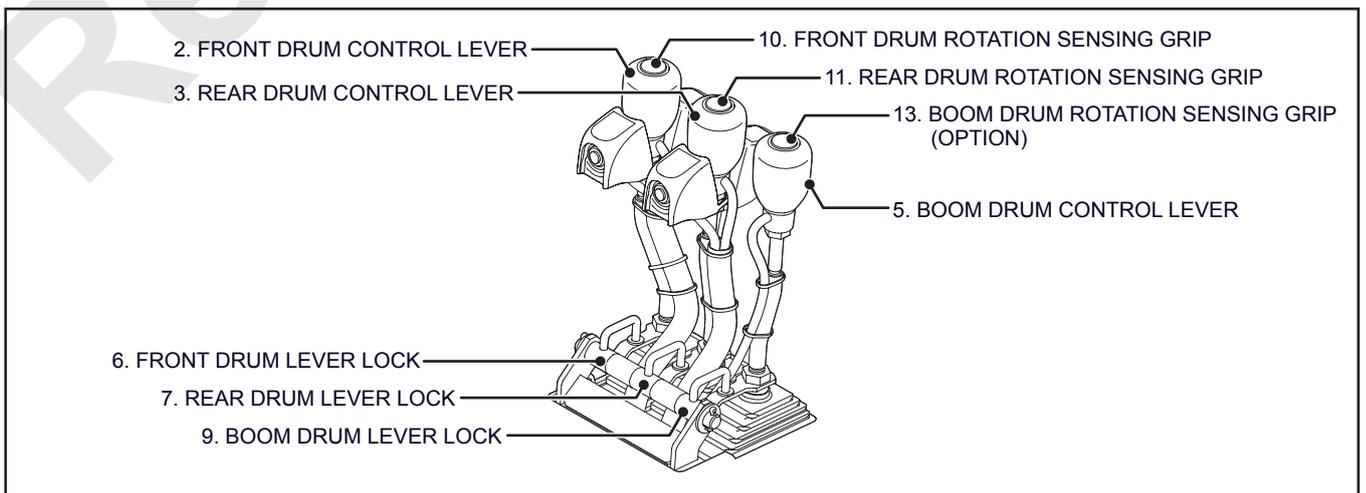
This article explains levers and pedals in the operator's cab.
