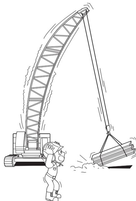
17. If the load strikes the boom or the boom hits a building or other object, the boom may collapse. Never let the load or any other object contact the boom.
