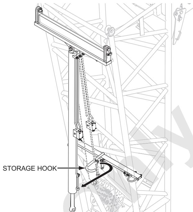
6. Lower the boom base to approximate 50 degrees and manipulate the control switch in the operator's cab to retract the cylinder.
