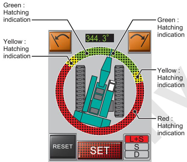
(B) If adjustment of area is not necessary, press **SET** (Set icon).
