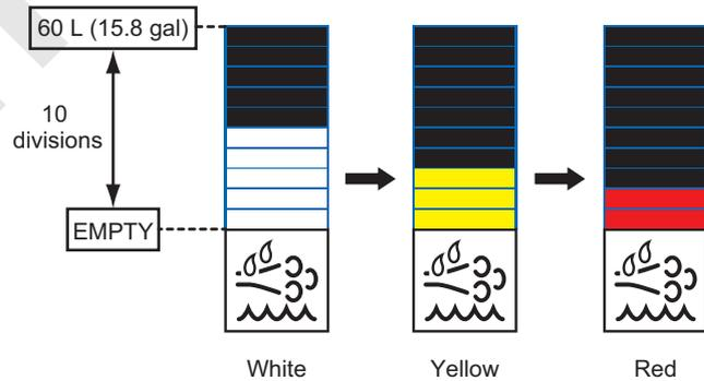
The bar gauge color changes from white to yellow when reaches to 3 blocks and changes to red when 2 blocks or less.
