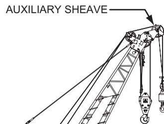
1. Align the holes of boom tip and auxiliary sheave frame.
