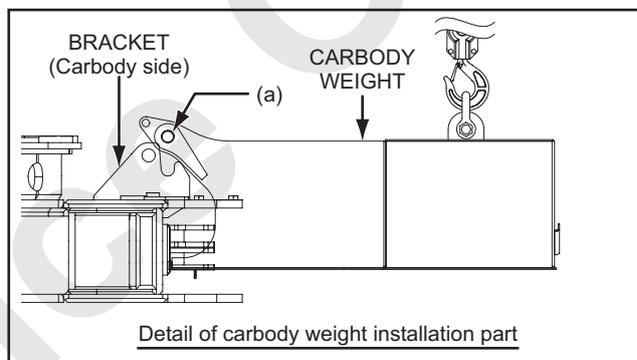
12. Lower the ratchet lever hoist and rest the carbody weight (a) portion to the carbody side hanging bracket.
