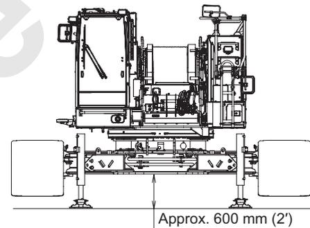
(20) Attach the slings to the left hand crawler frame and hold it with the self removal cylinder.
