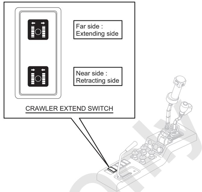
7. If the crawler still can't be retracted with the step 6 above performed due to bad ground condition, swing the upper machinery slowly to toward the side of the crawler desire to be retracted until the upper machine comes to right angle with the crawler.
