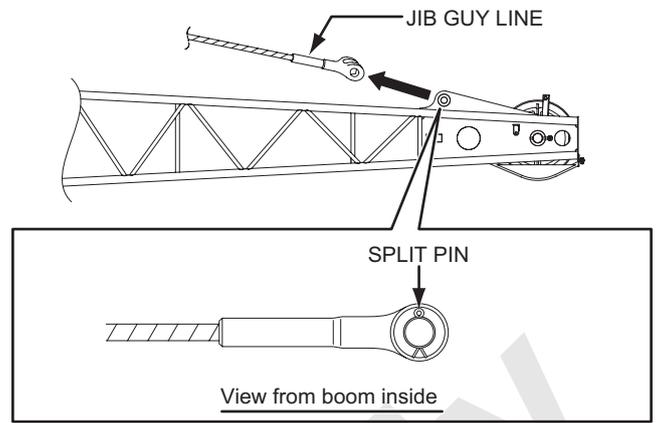
4. Remove the strut equalizer sheaves to take off the jib guy lines.
