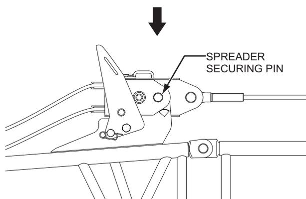
4. Disconnect the guy lines from the upper spreader. Put the connecting pins back to the upper spreader.
