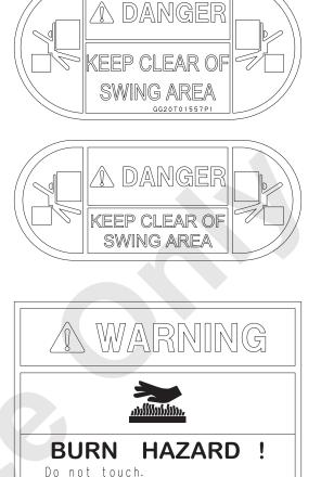
20. During engine running or straight after the engine is stopped, hydraulic oil tank, engine and muffler are hot.
