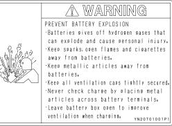
13. If accumulator is handled in wrong way, burns, loss of eyesight, explosion may be caused. Take extra care in handling accumulator. (Do not weld, flame cut, dispose or disassemble.)
