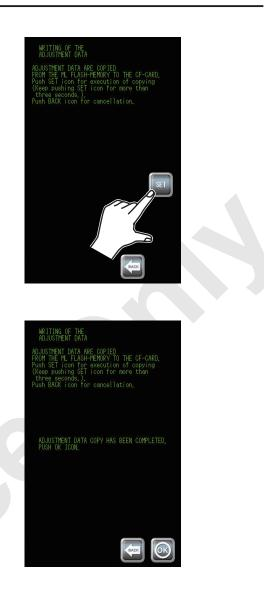
After execution, if error message as shown right is displayed, data card failure (including not enough insertion) is presumed. Re-insert the card and try again. By pressing , screen returns to the previous
