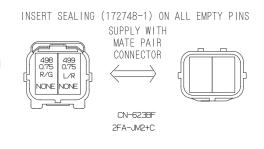
INSERT SEALING (172748-1) ON ALL EMPTY PINS
