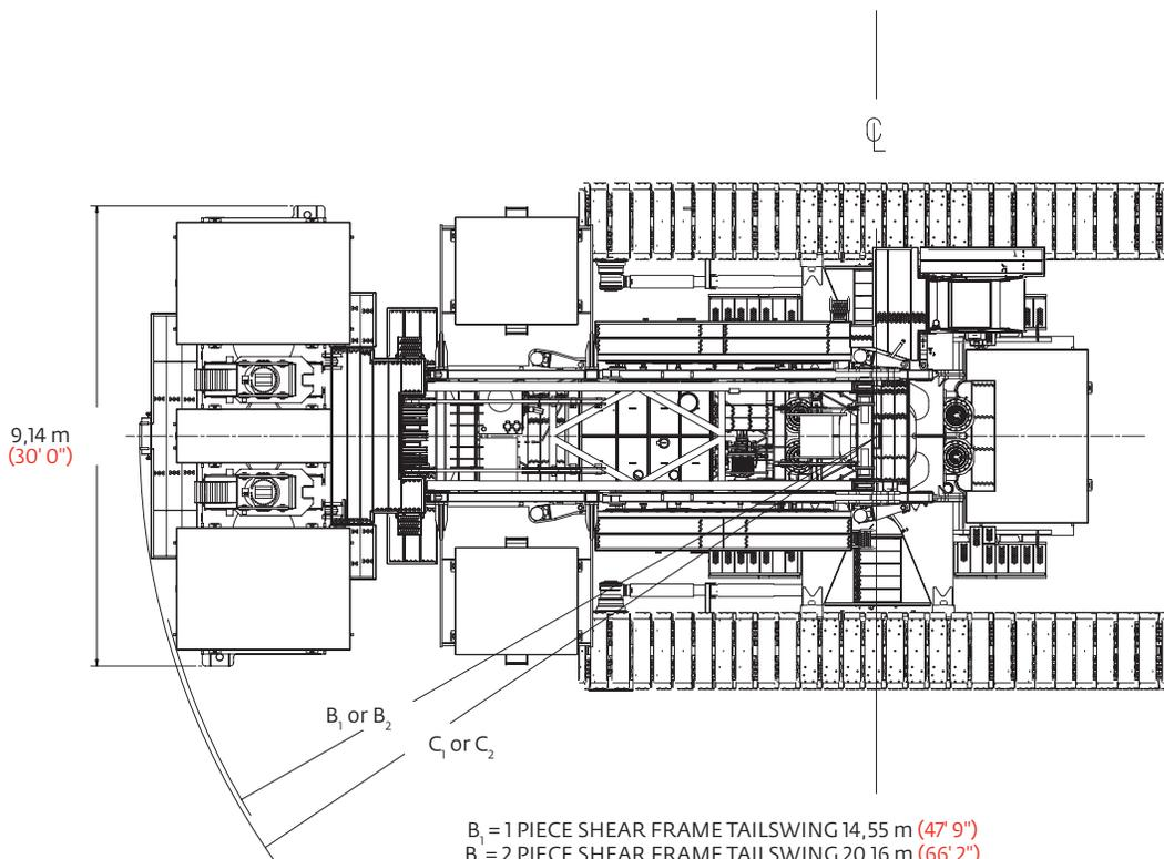
B<sub>1</sub> = 1 PIECE SHEAR FRAME TAILSWING 14,55 m (47' 9")
