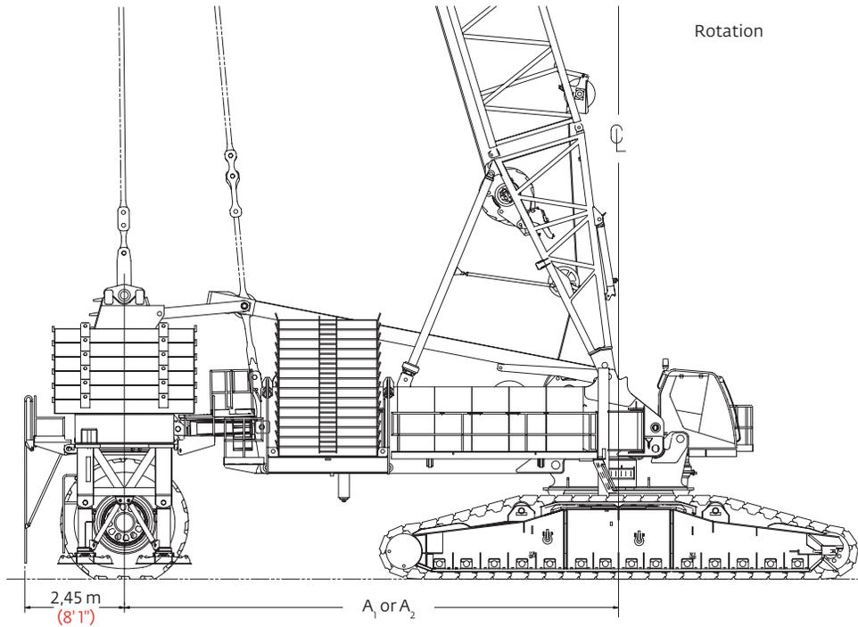
A<sub>1</sub> = 1 PIECE SHEAR FRAME 12,19 m (40' 0")
