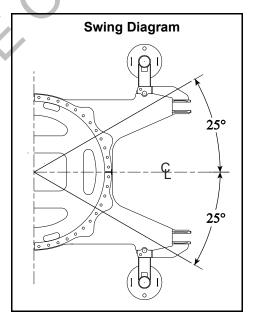
Operating Restrictions on Jacks with One Crawler Installed (four jacks with one crawler installed, OR two jacks with one crawler installed and on ground)
