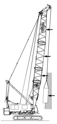
Backward stability is affected by wind on the front of the boom. This condition is especially dangerous when the boom is at or near the maximum angle when operating without load.
