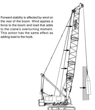
The wind's affect on the rear of the load increases load radius. This condition can result in an overload hazard, possibly causing the crane to tip or the boom to collapse.
