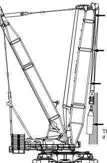
Backward stability is affected by wind on the front of the boom. This condition is especially dangerous when the boom is at or near the maximum angle when operating without load.
