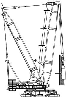
The wind's affect on the rear of the load increases load radius. This condition can result in an overload hazard, possibly causing the crane to tip or the boom to collapse.
