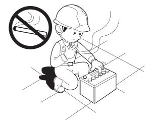
• Disconnect the battery cables during inspection and maintenance of electrical system.
