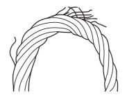
Bend rope sharply to expose breakage.
