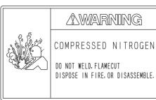
14. The accumulator is charged with high pressure nitrogen gas.
