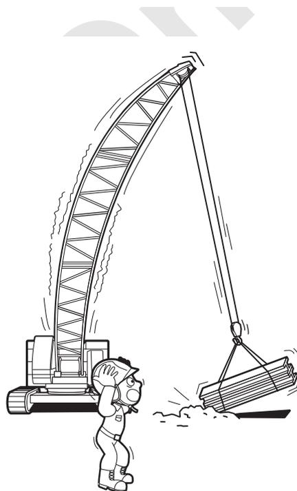
20. Trying to lift a load which is stuck, frozen or attached to something else may result in tipping, boom collapse or other damage. Be sure that loads are free before lifting.
