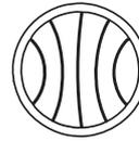
when the electrolyte level reaches the bottom of the sleeve, the electrolyte surface is swelled by surface tension, and the pole plates seen to be warp.
