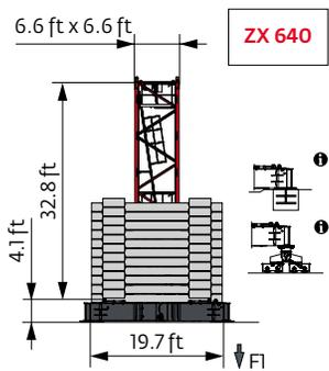
Note: When "ASCE" is noted in this data sheet it is referring to 115 mph Wind Zone, Exposure B, Design Wind Speed = 98 mph. See back cover for design wind speed calculations.
