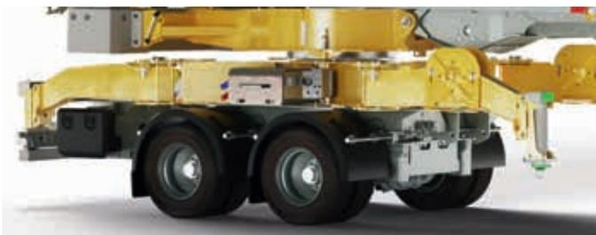
dual steering axle  $+20^{\circ}/-20^{\circ}$
