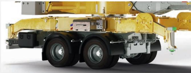
Dual steering axle  $+20^{\circ}/-20^{\circ}$
