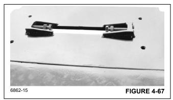
**NOTE:** Installation of the extend cable anchor assembly will require the use of a bolt longer than the permanent bolt. The weight of the five extend cables and anchor assembly will make the installation of the anchor assembly extremely difficult without use of a longer bolt. (Refer to Figure 4-68).
