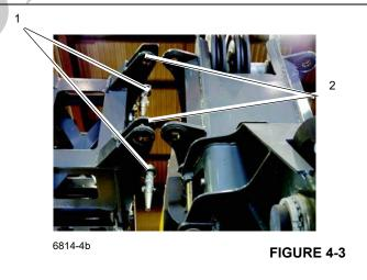
**NOTE:** Prior to Step 6, before removing the hitch pin (3), ((Figure 4-4)), make sure that the boom extension is attached to the right side boom nose attachment lugs with the pins and that the pins are secured.
