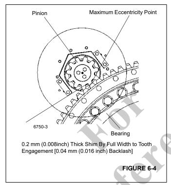
Orient ring gear to the point of max eccentricity ("high point"). Position swing drive so that pinion is centered within cutout in base plate and the motor ports face towards the outboard side as shown in (Figure 6-4).
