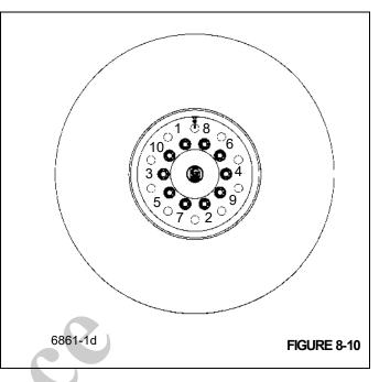
torque every 800 km (500 mi) thereafter. An alternative to re-torquing after 80 km (50 mi) is to run the machine in large figure 8's six or seven times and then re-torque the lug nuts.
