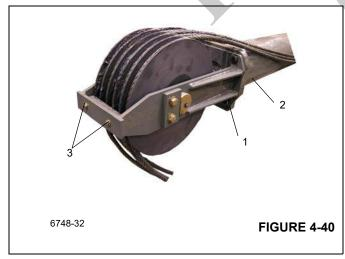
**5.** Mark **BOTH ENDS** of the five extend cables (Figure 4-43).
