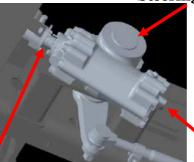
Left turn relief Screw in to decrease travel Screw out to increase travel Right turn relief Screw in to decrease travel Screw out to increase travel
