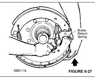
5. Rotate the bottom brake shoe to relieve tension on the retaining springs. Remove the springs and brake shoes.
