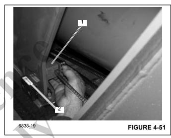
8. Slide the fly section into the outer mid section until the wear pad adjustment is accessible though the access plate (2), (Figure 4-51) on top of the outer mid section.
