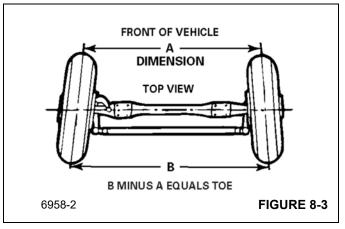
0.794mm (1/32 inch) ± 0.794mm (1/32 inch) for Loaded vehicle.
