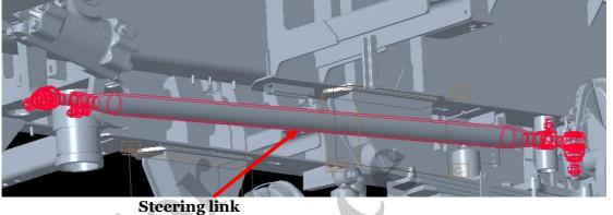
• Steering stops should be set to provide 1.00 in. (25.4 mm) of clearance to closest object for any tire.
