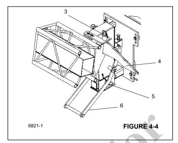
Extend the boom approximately 51 to 64 cm (20 to 25"). Make certain that the boom extension stowage lugs clear the guide pins (1), (Figure 4-5) and ramp (4), (Figure 4-4) on the front and rear stowage brackets.
