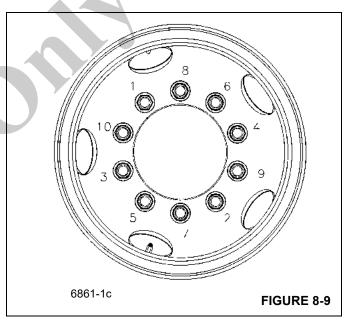
NOTE: Do not lubricate the wheel studs or lug nuts. On aluminum wheels, lubricate only the pilot or hub pads with synthetic lubricant containing Teflon. Do not lube the face of the wheel or rim.
