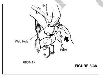
5. Install the slack adjuster. Reference *Automatic Slack Adjuster*, page 8-40.
