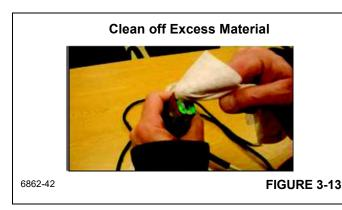
Make sure that each socket has material. The towel with excess material can be used to fill empty terminal sockets as shown in (Figure 3-14).
