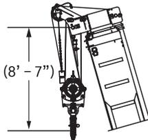
DIMENSIONS ARE FOR LARGEST FURNISHED HOOK BLOCK & HEADACHE BALL, WITH ANTI-TWO BLOCK ACTIVATED.
