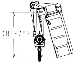
DIMENSIONS ARE FOR LARGEST FURNISHED HOOK BLOCK & HEADACHE BALL, WITH ANTI-TWO BLOCK ACTIVATED.
