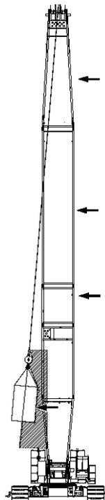
The wind's affect on the side of the load can cause the load to swing out past the boom hinge pin.
