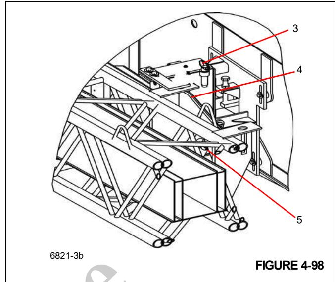
8. Be sure that the sliding portion (4), (Figure 4-98) of the rear storage bracket is in the “OUT” position and secured in place with retaining pin(s) (5), (Figure 4-98) before Step 9.
