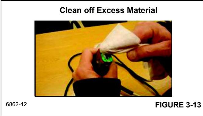
4. Make sure that each socket has material. The towel with excess material can be used to fill empty terminal sockets as shown in (Figure 3-14).
