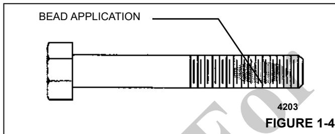
1. Apply a bead perpendicular to the thread, several threads wide, in the approximate area of threaded engagement (Figure 1-4).
