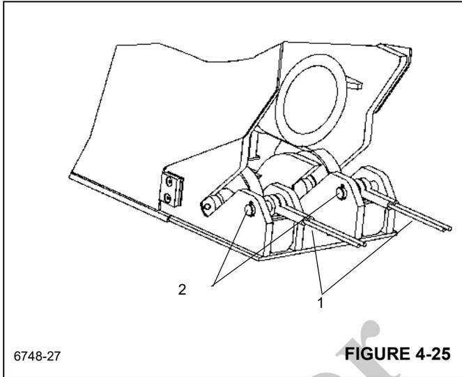
13. If necessary, remove the two bolts securing the bottom wear pad to the inner mid section. Remove the wear pad.
