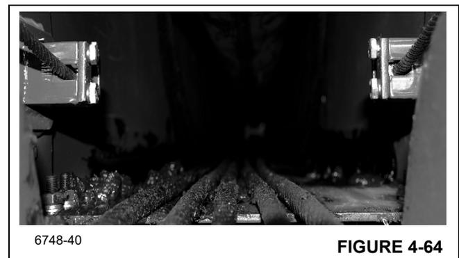
5. Pass the threaded end of the fly retract cables down through the bottom of the fly section. Lay the cables out toward the nose end of the fly section.
