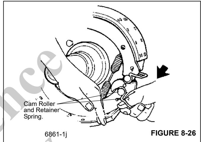
2. Lift the top brake shoe and pull on the roller retaining clip and remove the upper cam roller.
