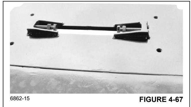
**NOTE:** Installation of the extend cable anchor assembly will require the use of a bolt longer than the permanent bolt. The weight of the five extend cables and anchor assembly will make the installation of the anchor assembly extremely difficult without use of a longer bolt. (Refer to Figure 4-68).
