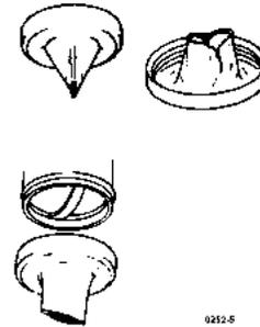
Vacuator valves are designed to expel loose dust and dirt from the air cleaner body automatically, thus lengthening the element service life. The valve lips must point straight down and be kept free from debris to operate effectively. Mud and chaff can lodge in these lips periodically and hold them open during engine operation.
