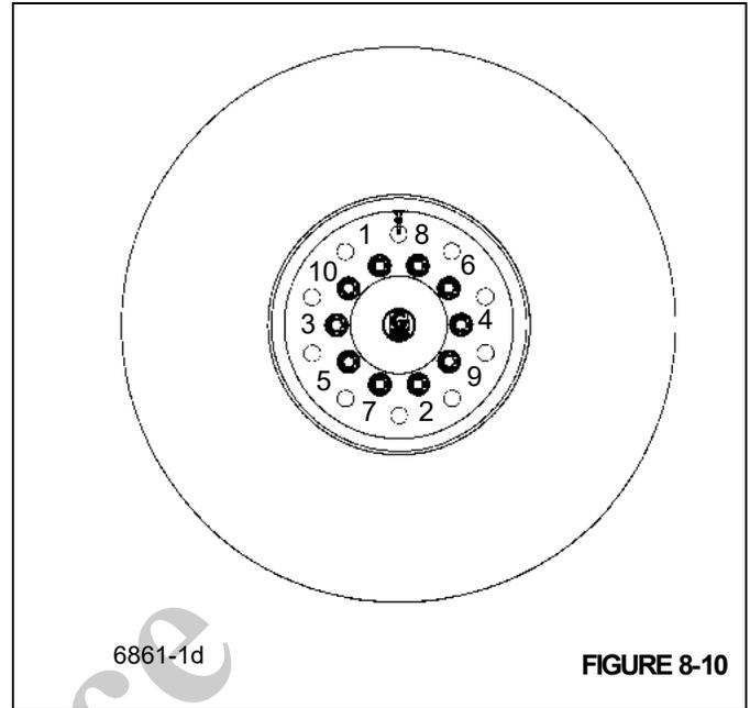
torque every 800 km (500 mi) thereafter. An alternative to re-torquing after 80 km (50 mi) is to run the machine in large figure 8's six or seven times and then re-torque the lug nuts.
