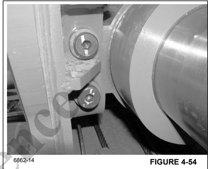
14. Remove the block of wood holding the Telescope Cylinder.
