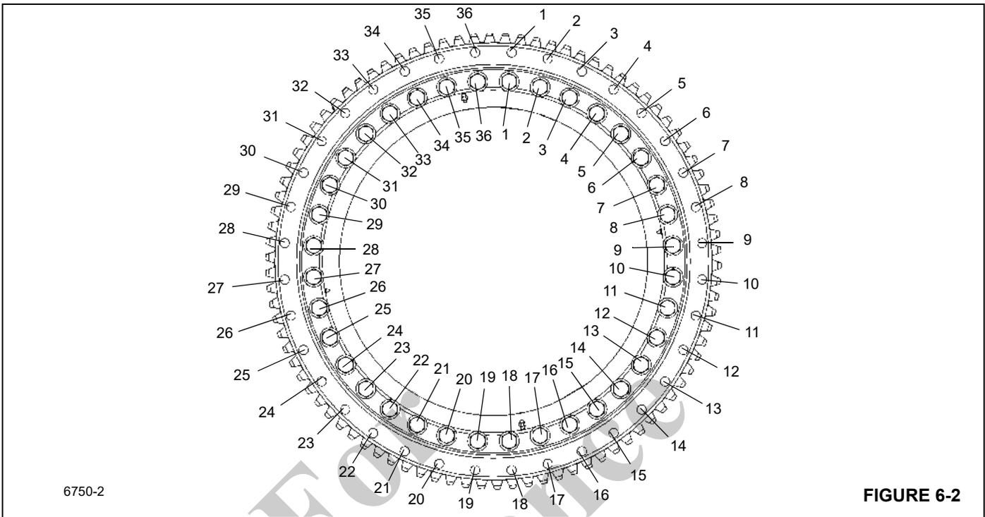
The inner race of the bearing is secured to the turntable by 36, 1 inch, grade 8 bolts. The outer race of the bearing is secured to the carrier frame by 36, 7/8 inch, grade 8 bolts.
