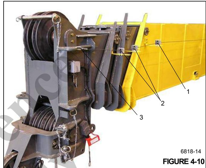
4. Chain the Fly, Outer Mid and Inner Mid sections together as shown in Figure 4-11. This will prevent the inadvertent or unexpected extension of these sections during the boom disassembly.
