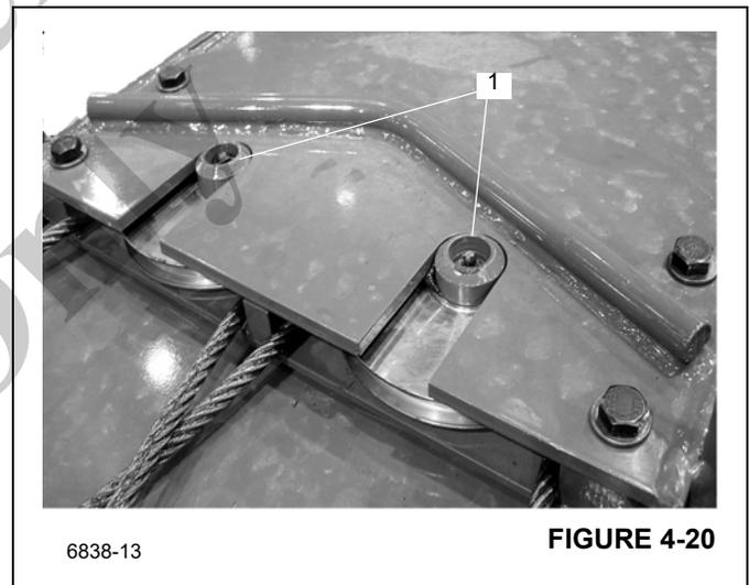
4. At the lower front of the inner mid section, remove the bolts securing the fly retract cable anchor plates (1), (Figure 4-21). Remove the cable locknuts and the anchor plates from the cables.
