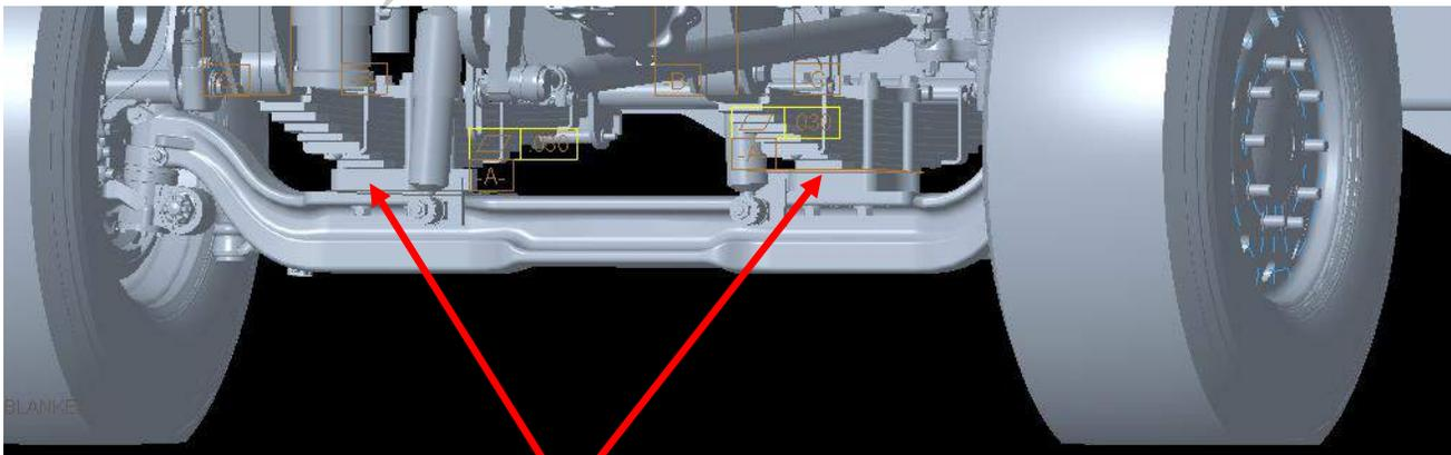
**Install shims between the spring assemblies and shock plates.**
