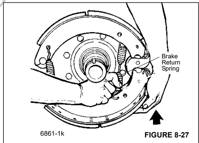
5. Rotate the bottom brake shoe to relieve tension on the retaining springs. Remove the springs and brake shoes.
