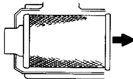
2. Inspect all parts of the intake system and air cleaner. Be sure to clean the sealing surface of the outlet tube and the inside of the outlet tube.
