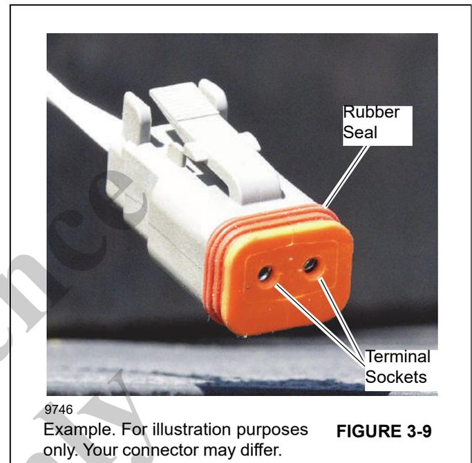
4. Use a clean towel to remove excess grease from the surface of the connector, and wipe grease into the terminal sockets (Figure 3-9).
