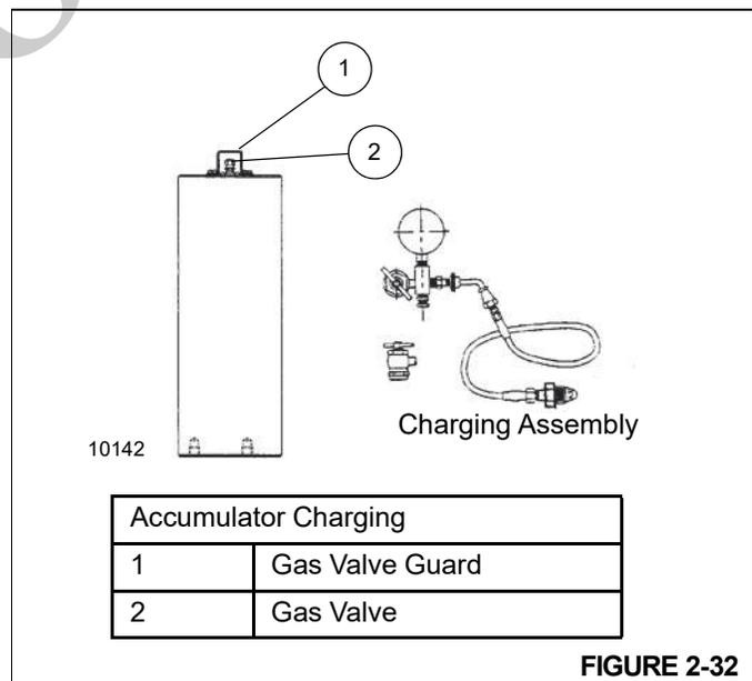
**Checking the Service Brake Accumulator Pre-charge**
