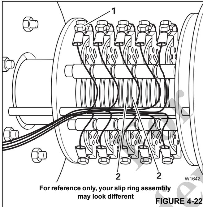
5. Remove visible dirt on the slip rings (2, Figure 4-22) with a clean, lint-free cloth.
