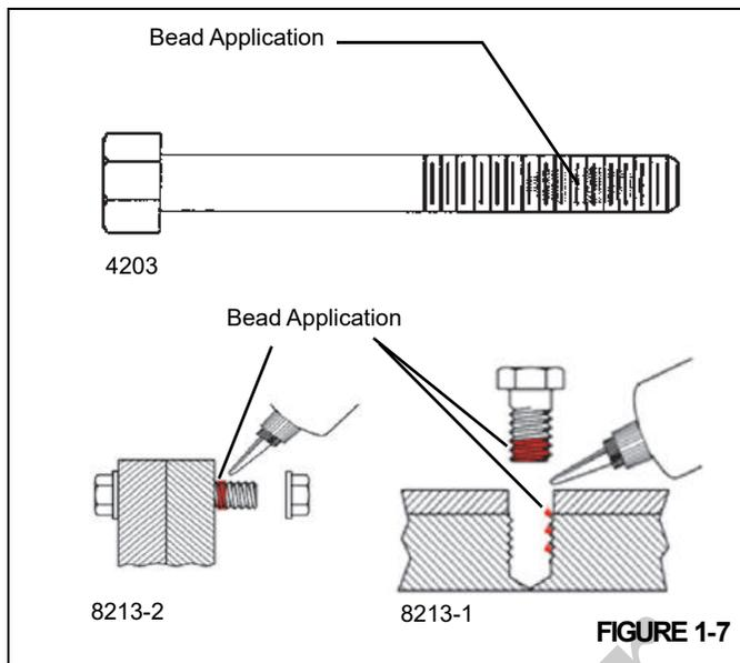
3. After application and engagement of mated threads, fixturing will occur within five (5) minutes. Time required to achieve full strength is 24 hours.
