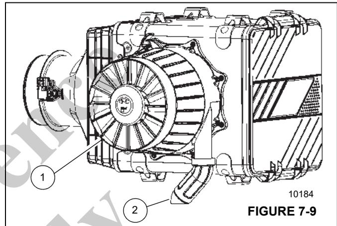
**FIGURE 7-9****Evacuator Valve**
