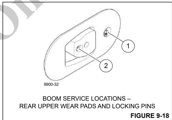
6. While in the horizontal position, first retract Tele 4, and then retract and extend Tele 5 several times to make sure that grease is properly distributed.
