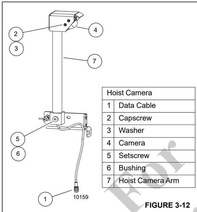
2. Remove capscrews (2), washers (3), and camera (4) from hoist camera arm (7).
