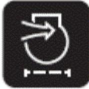
The condition of the air filter is monitored by a sensor. The degree of contamination is determined by measuring the resistance to air flow through the filter. If the maximum permissible flow resistance is reached, the air filter indicator light is illuminated on the SENCON Air filter. A warning tone also sounds. Check and clean the air filter immediately.
