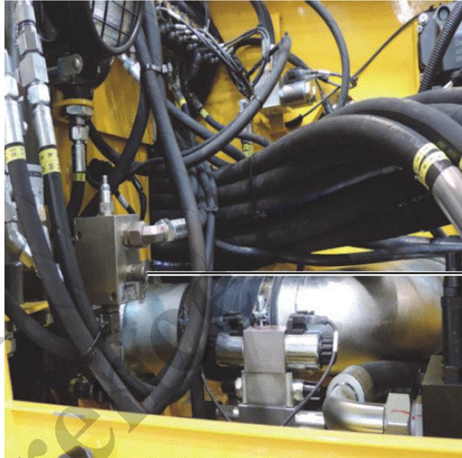
*Fig. 24: Pressure accumulator measurement connection*
