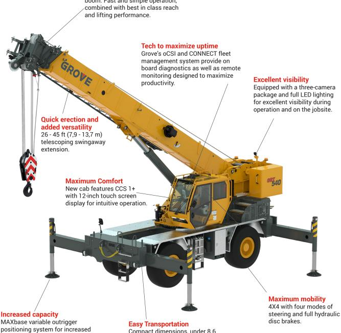
positioning system for increased lift capacities and easy access to any jobsite.
