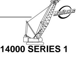
**OPERATING RADIUS:** Operating radius is horizontal distance from axis of rotation to center of gravity of freely suspended load./
