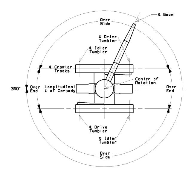
These lines determine limiting position of any load for operation within working areas indicated.
