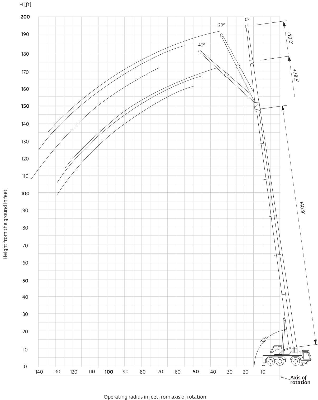
Tip heights shown in the working range diagram do not consider loaded boom deflection.
