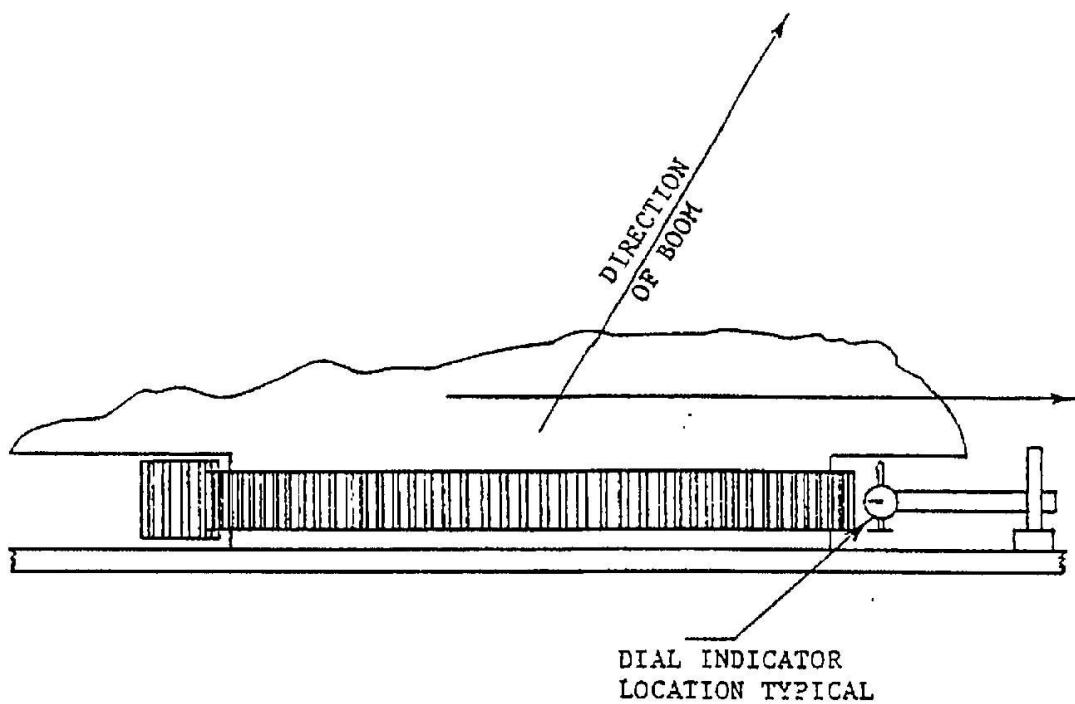
**Measurement of Turntable Bearing Vertical Movement**
