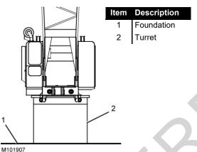
Figure 2-5. Turret-Mounted Crane
