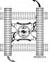
Figure 3-21. Counter-Rotate Left
