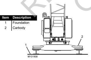
Figure 2-6. Carbody-Mounted Crane
