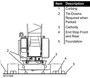
Figure 2-8. Crawler-Mounted Crane
