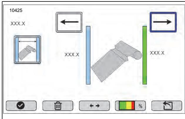
1. Move the crane boom to the desired boom radius (it appears on the display screen).
