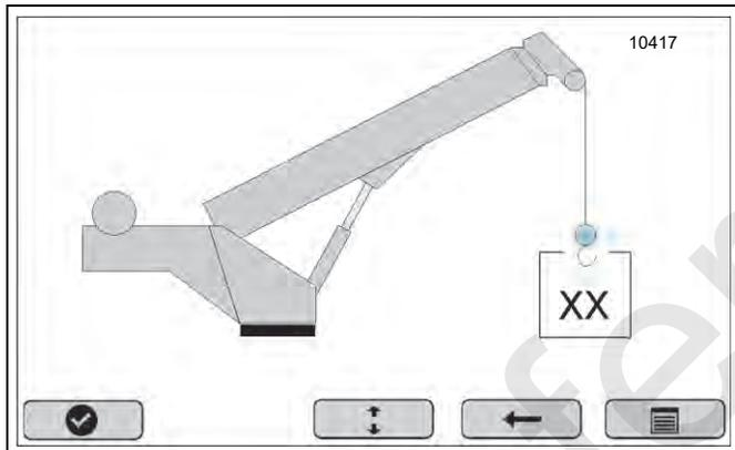
After hoist selection, use the up and down arrows to change reeving from 1 part line up to 7 parts line on Screen 8.
