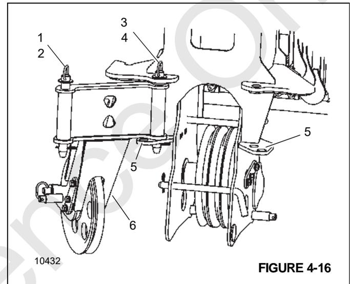
1. Remove the cotter pin (2 or 4, Figure 4-16) and pin (1 or 3) from one side of the auxiliary boom nose (6).
