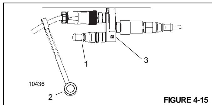
4. Remove the resistor (1, Figure 4-15) from the cap (2). Install the resistor in splitter port B (3).
