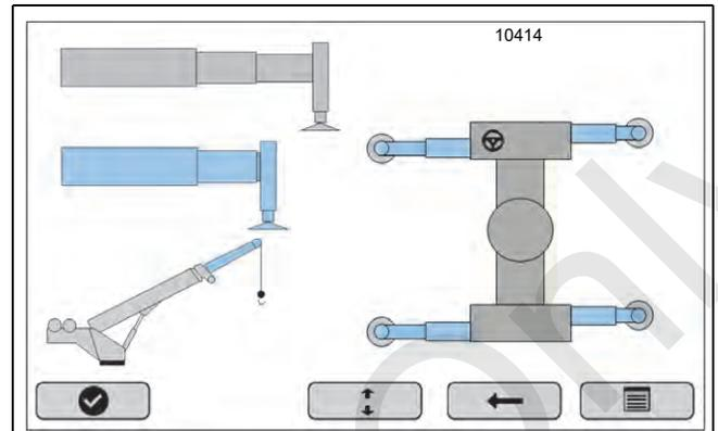
If the user attempts to select the check mark before Fully Extended, 75%, or 50% Extended condition is met, the check mark button is colored RED when depressed and the user can override the setup using the arrow keys.
