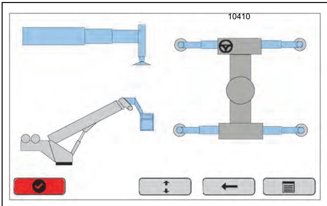
If the user attempts to select the check mark before the Fully Extended condition is met, the check mark button is missing. The user can override the setup using the arrow keys and the check mark.
