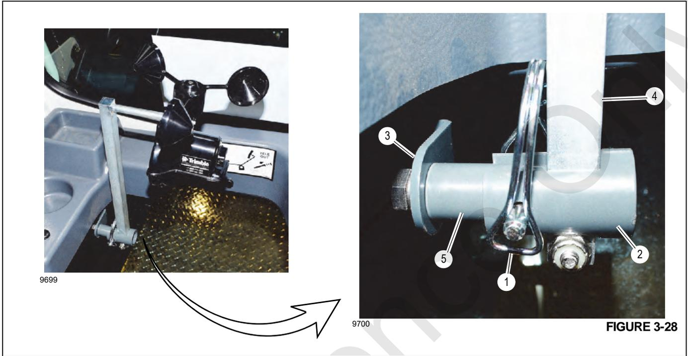
2. In the cab, remove the safety pin (1, Figure 3-28) and bushing (2) from the anemometer stowage bracket (3).
