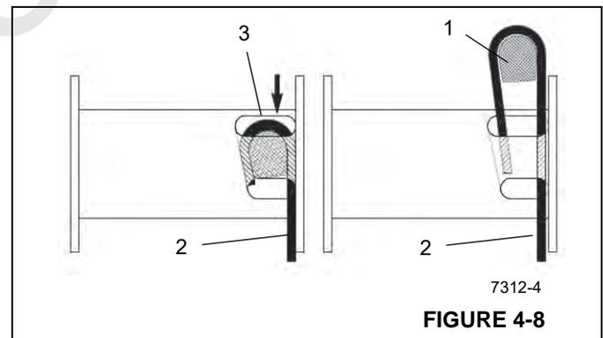
4. Position the anchor wedge in the drum slot; pull firmly on the free end (2) of the rope to secure the wedge.
