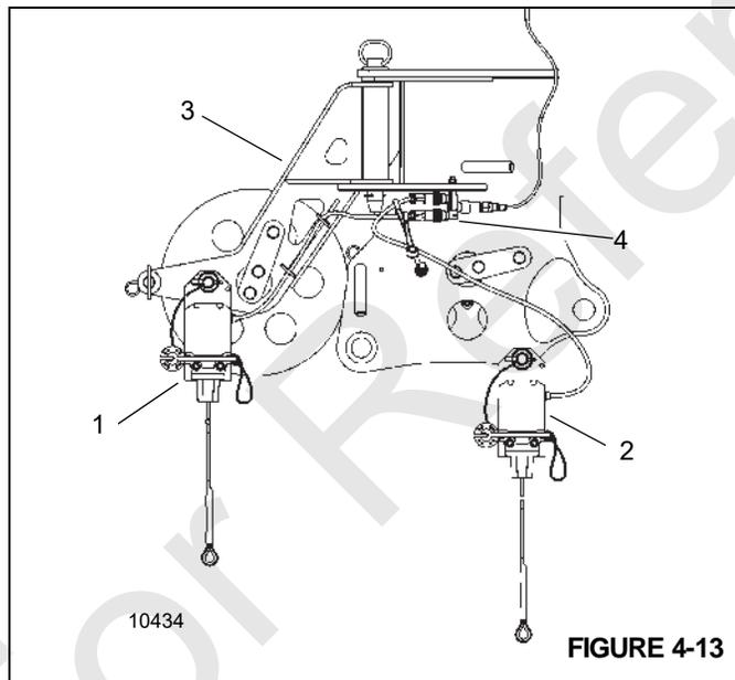
1. Install the auxiliary boom nose (3). For more information, see *Installing the Auxiliary Boom Nose*, page 4-21.
