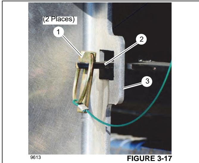
**Stowing the Ladder on Rear Bumper for Transport**
