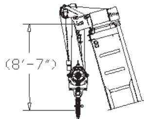
DIMENSIONS ARE FOR LARGEST FURNISHED HOOK BLOCK & HEADACHE BALL, WITH ANTI-TWO BLOCK ACTIVATED.
