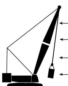
Backward stability is affected by wind on the front of the boom and luffing jib. This condition is especially dangerous when the boom and/or luffing jib is at or near the maximum angle when operating without load.
