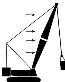
Forward stability is affected by wind on the rear of the boom and luffing jib. Wind applies a force to the boom, luffing jib, and load that adds to the crane's overturning moment. This action has the same effect as adding load to the hook.
