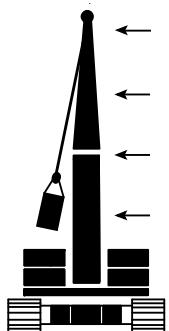
Boom and luffing jib strength is affected the most when the wind acts on the side of the boom and luffing jib.
