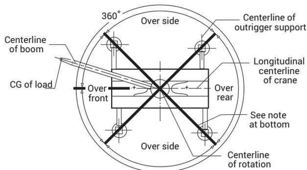
Diagram for lifting on tires
