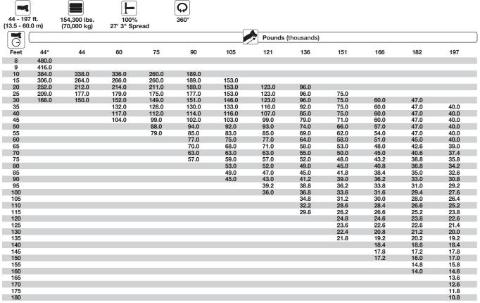
\* Over rear only, 27'10" x 18'8" outrigger base. Lifting capacities greater than 350,000 lbs (160,000 kg) require additional equipment.
