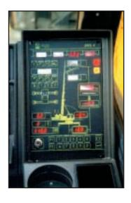
electronic load moment indicator that operates in conjunction with ECOS continuously displaying crane configuration and load moment data
