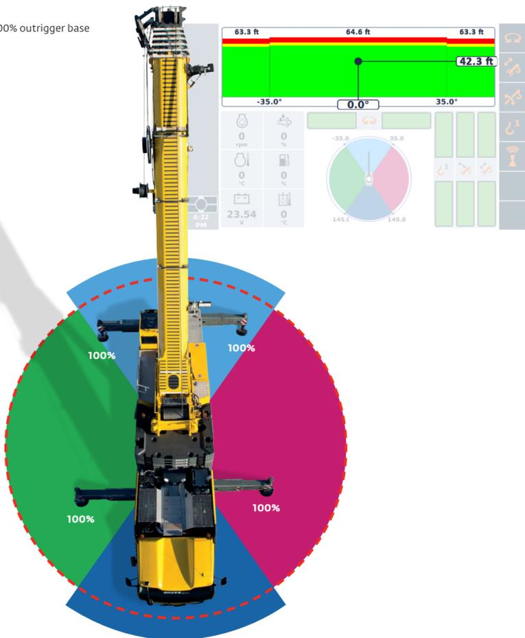
MAXbase calculations improve even symmetrical outrigger positioning. The four-sector calculation formula allows an increase to 360° charts by more specifically defining your stability limitations and taking advantage of them.
