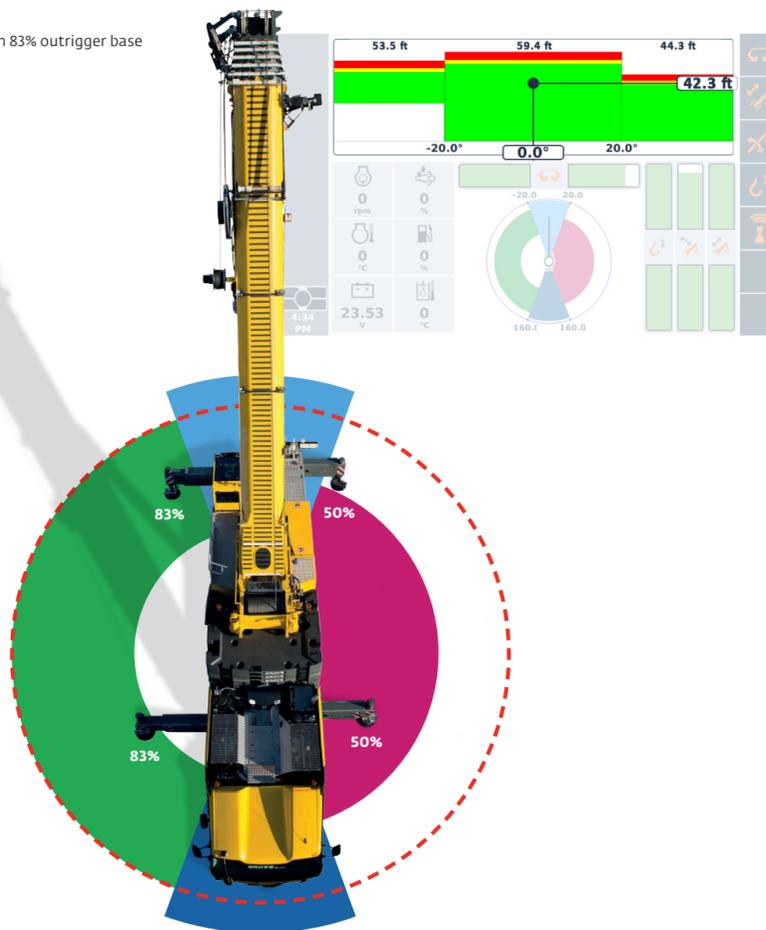
MAXbase, allows the outriggers to be controlled, symmetrically right and left or front and rear. This provides better access to tighter job sites and closer positioning to the lift. Reduce transport costs by leaving costly jibs and counterweight at the yard.
