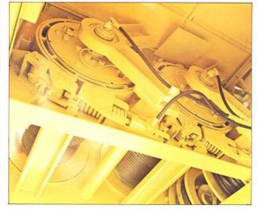
FOUR SECTION HYDRAULIC OIL PUMPS - Two dual section gear type pumps driven from front of carrier engine have manual pump disconnect operated from carrier cab for efficient road travel.
