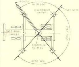
NOTE: Bold lines determine the limiting position of any load for operation within working areas indicated.
