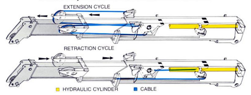
EXTENSION CYCLE - As the mid-section is extended by the telescope cylinder, the fly section is pulled out of the mid-section in direct proportion by a % in. (22mm) cable. The extension cable has a safety factor of 3.5 to 1 (6 to 1 with international version and 11/s in. (29mm) dia. cable) and is attached with threaded connections at base section and retained on either side of the sheave segment by swaged collars. This prevents the boom from retracting should the cable break.
