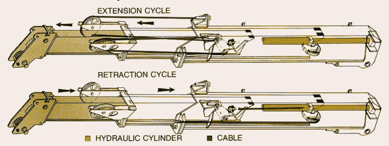
the telescope cylinder, the fly section is extended by the mid-section in direct proportion by a % in. (22mm) cable. The extension cable has a safety factor of 3.5 to 1 (6 to 1 with international version and 11/8 in. (29mm) dia. cable) and is attached with threaded connections at base section and retained on either side of the sheave segment by swaged collars. This prevents the boom from retracting should the cable break.
