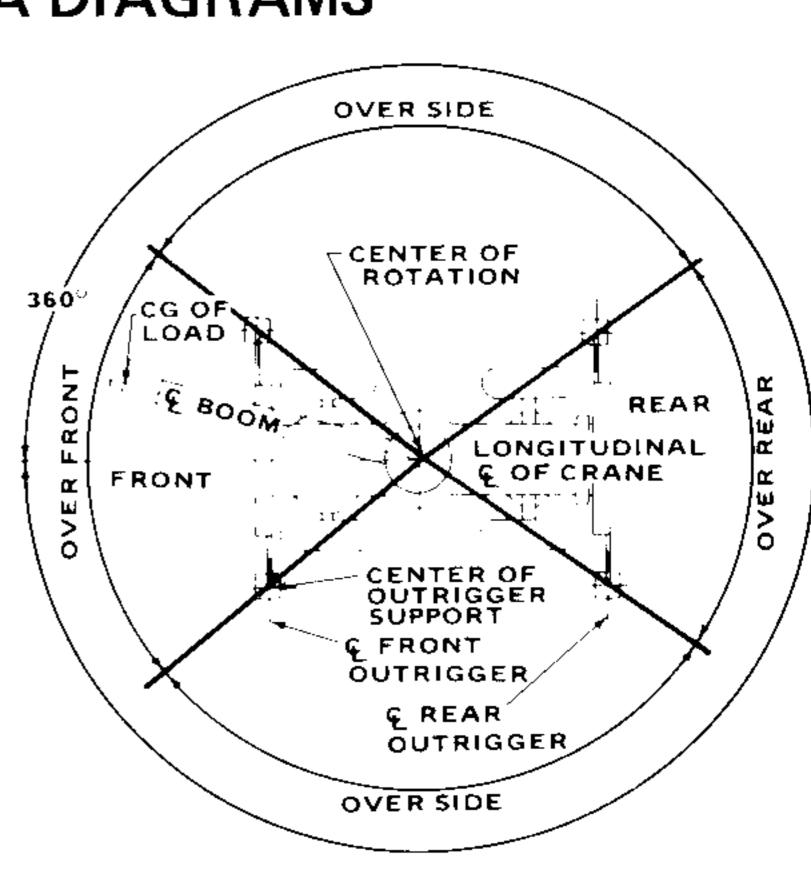
NOTE: BOLD LINES DETERMINE THE LIMITING POSITION OF ANY LOAD FOR OPERATION WITHIN WORKING AREAS INDICATED.
