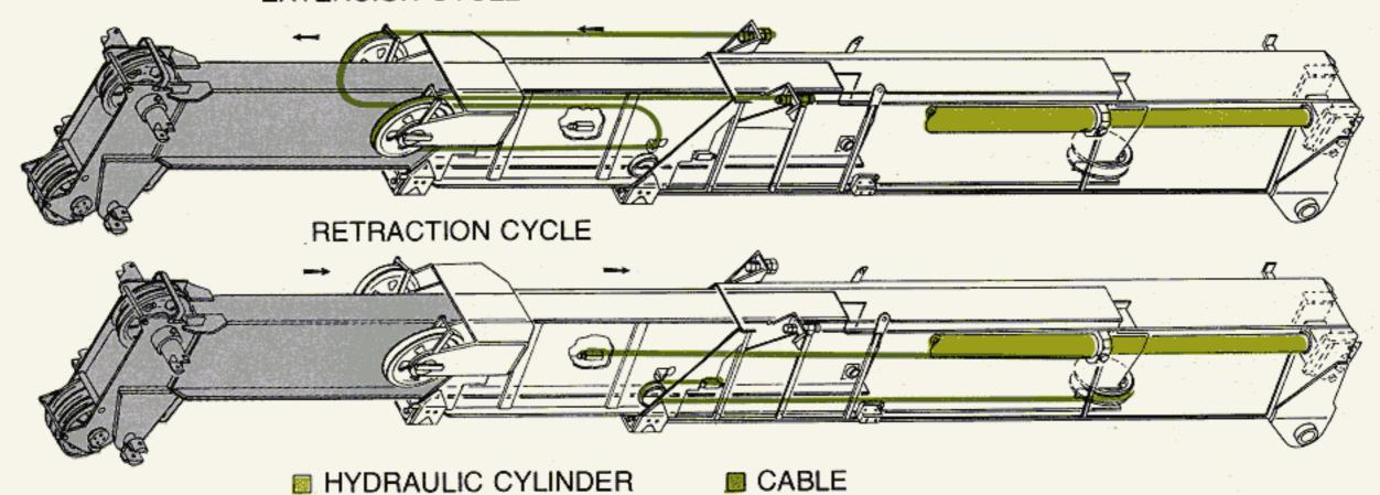
the telescope cylinder, the fly section is extended by the telescope cylinder, the fly section is pulled out of the mid-section in direct proportion by a 11/8 in. cable. The extension cable has a safety factor of better than 5 to 1 and is attached with threaded connections at base section and retained on either side of the sheave segment by swagged collars. This prevents the boom from retracting should one of the cables break.
