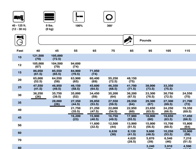
Minimum boom angle (deg.) for indicated length (no load)
